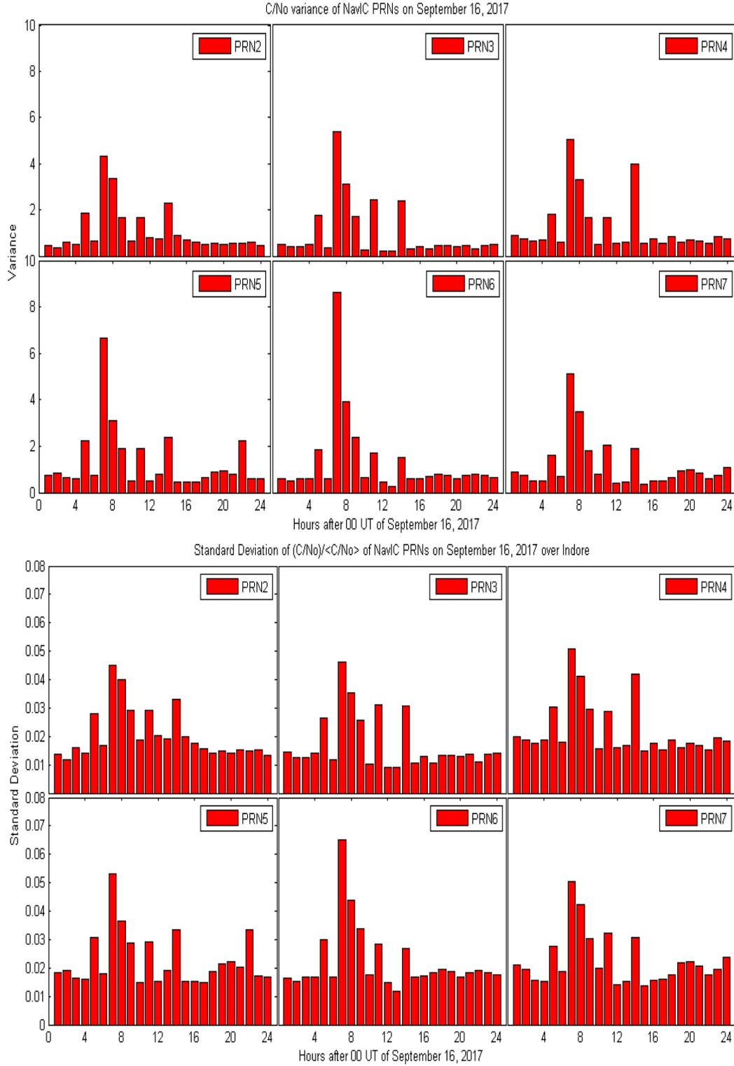
**Figure 10.** The hourly binned variance plots (top panel) of  $C/N_0$  and the corresponding standard deviation plots (bottom panel) of  $\frac{C/N_0}{\langle C/N_0 \rangle}$  for all PRNs of NavIC on September 16, 2017 over Indore.
