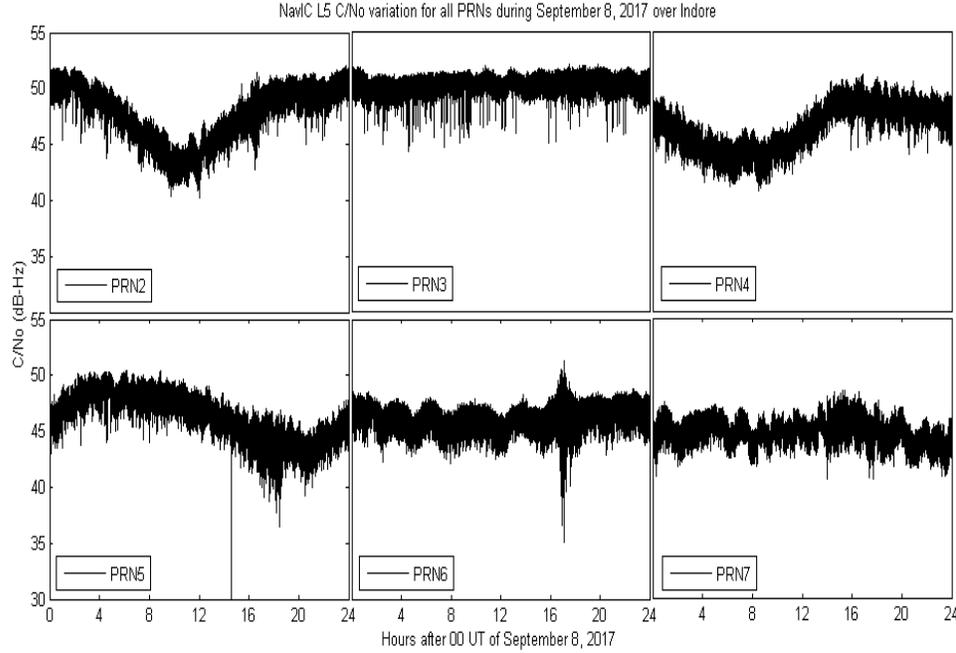
**Figure 1.** The  $C/N_o$  (dB-Hz) variation during the disturbed day of September 8, 2017, as observed by L5 signal of NavIC satellite PRNs 2-7 over Indore. It is to be noted here that  $LT=UT+05:30h$ .
