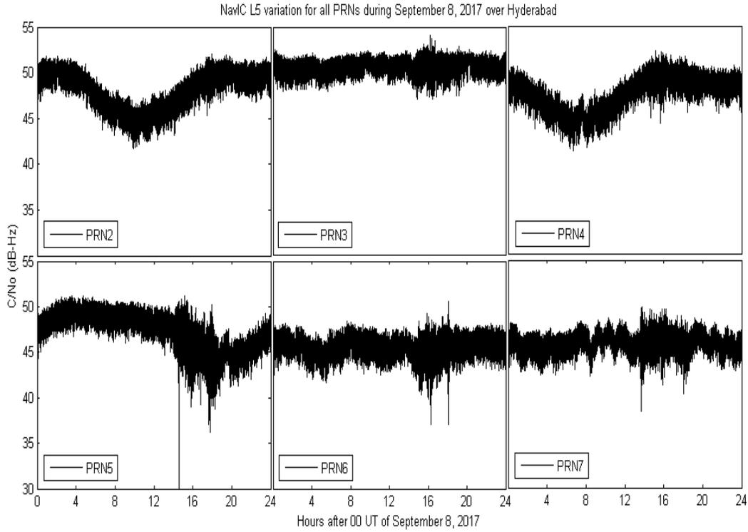
**Figure 6.** The  $C/N_o$  (dB-Hz) variation during the disturbed day of September 08, 2017, as observed by L5 signal of NavIC satellite PRNs 2-7 over Hyderabad.
