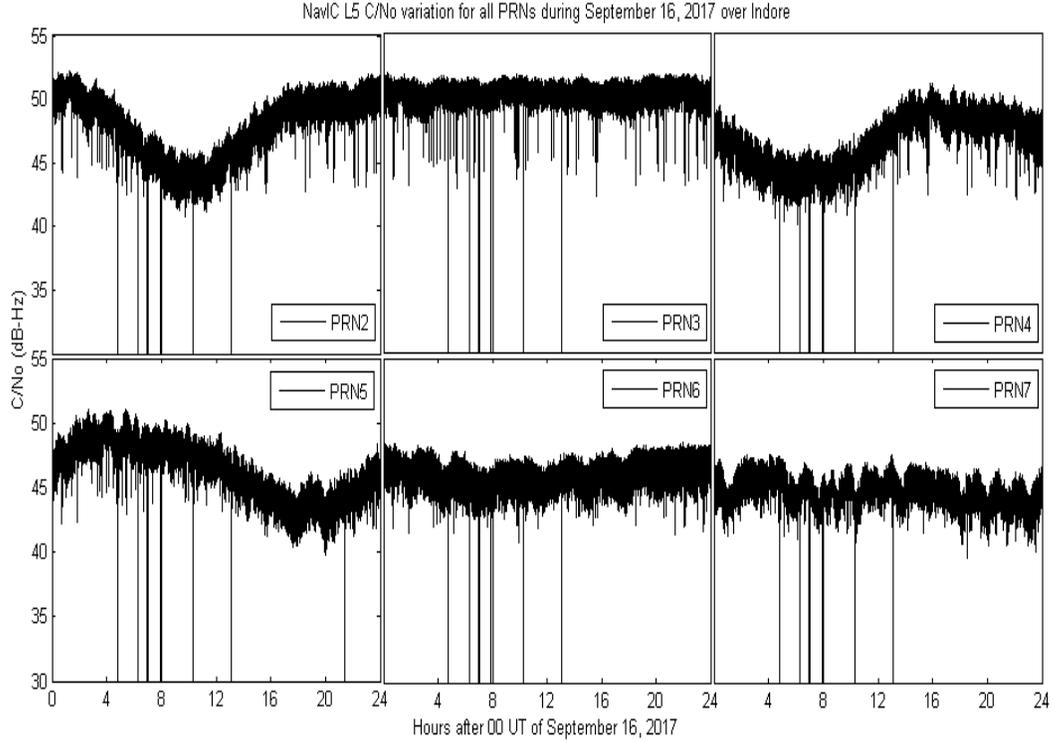
**Figure 9.** The  $C/N_o$  (dB-Hz) variation during the entire quiet day of September 16, 2017 over Indore, as observed by L5 signal of NavIC satellite PRNs 2-7.
