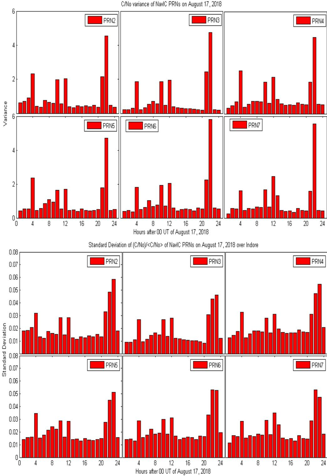
**Figure 13.** The hourly binned variance plots (top panel) of  $C/N_0$  and the corresponding standard deviation plots (bottom panel) of  $\frac{\langle C/N_0 \rangle}{\langle C/N_0 \rangle}$  for all PRNs of NavIC on August 17, 2018 over Indore.
