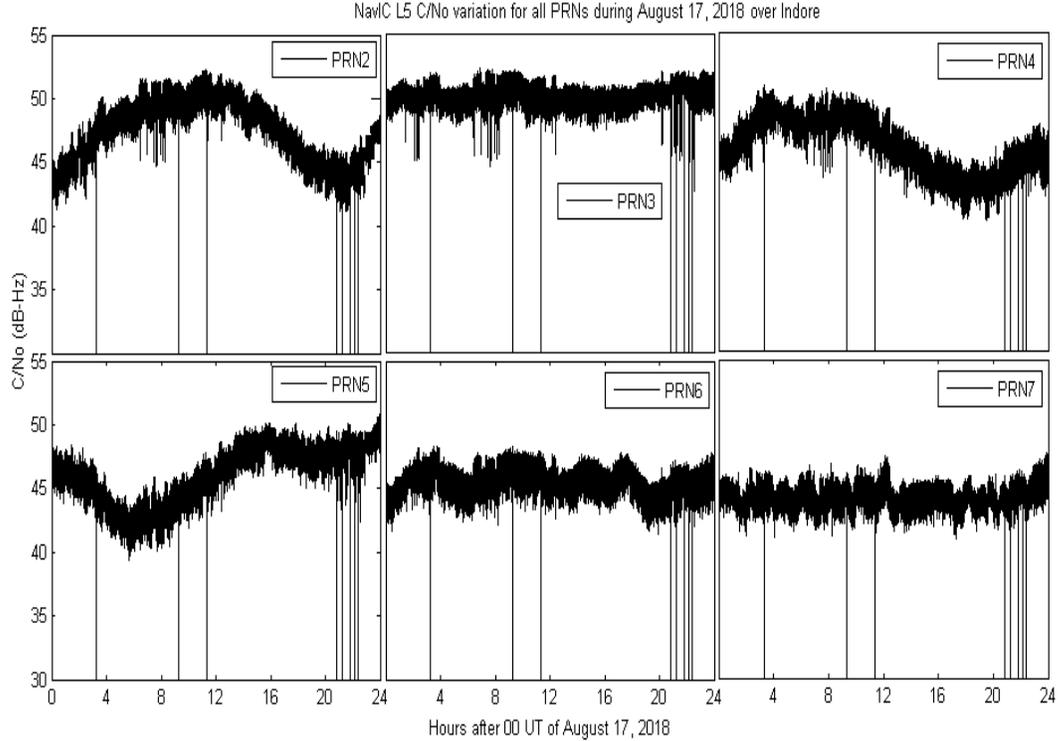
**Figure 12.** The  $C/N_o$  (dB-Hz) variation during the entire day of August 17, 2018 over Indore, as observed by L5 signal of NavIC satellite PRNs 2-7.
