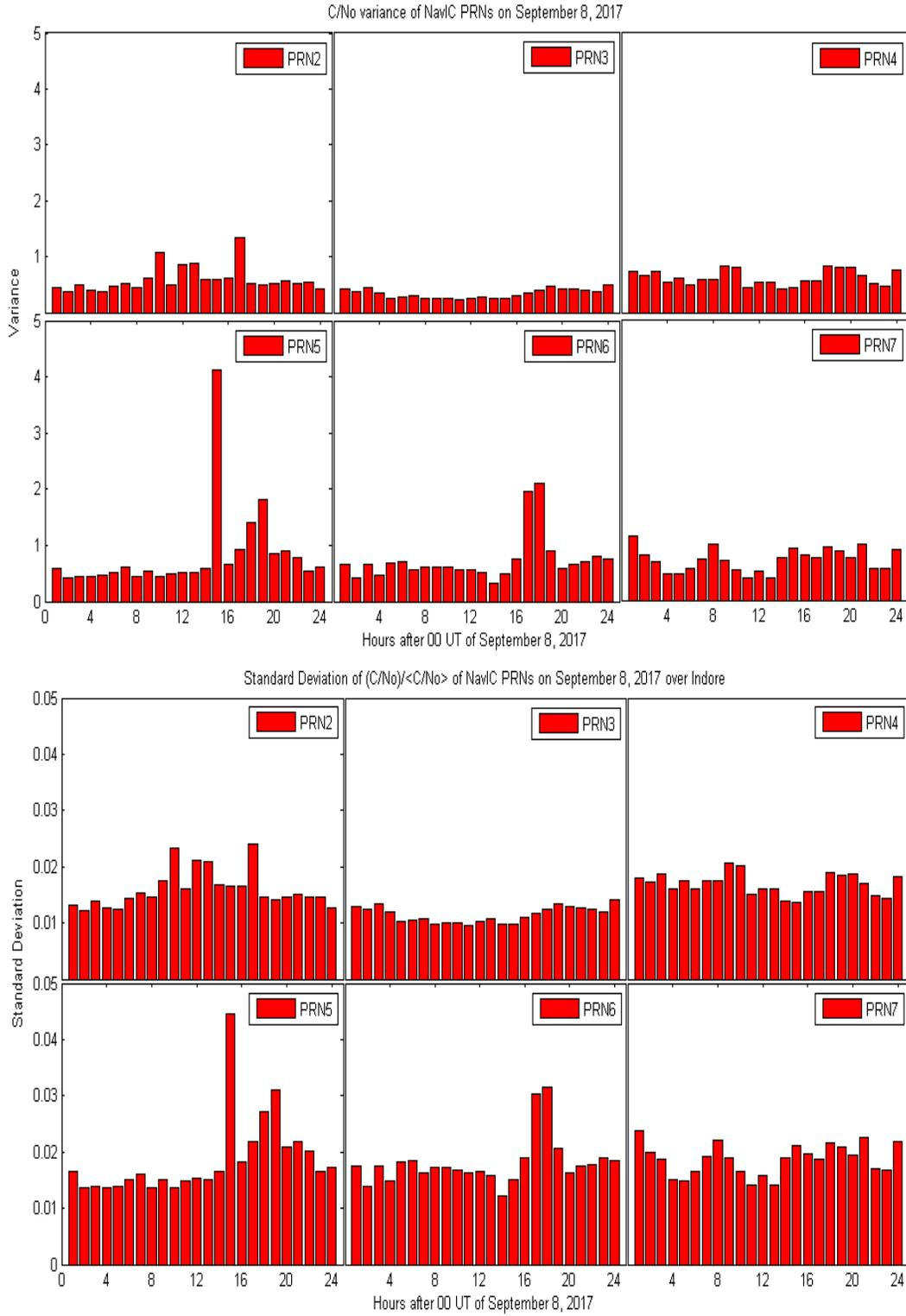
**Figure 2.** The hourly binned variance plots (top panel) of  $C/N_0$  and the corresponding standard deviation plots (bottom panel) of  $\frac{C/N_0}{\langle C/N_0 \rangle}$  for all PRNs of NavIC on September 8, 2017 as observed from Indore.
