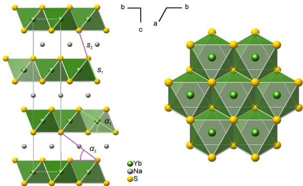
FIG. 1. Crystal structure of  $\text{NaYbS}_2$  in  $R\bar{3}m$  viewed along  $a$  (left) and section of an  $\text{YbS}_6$  layer (right). The unit cell is depicted in light grey. Interlayer sulfur - sulfur distances  $s_1$  (light green) and  $s_2$  (lavender) as well as the torsion angles  $\alpha_1$  (light green) and  $\alpha_2$  (lavender) of the  $\text{YbS}_6$  and  $\text{NaS}_6$  octahedra respectively are highlighted; see text for details.
