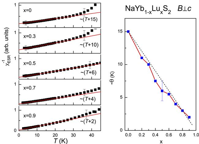
FIG. 6. Temperature dependence of the reciprocal ESR intensity  $\chi_{\text{ESR}}^{-1}$  for various  $x$  in  $\text{NaYb}_{1-x}\text{Lu}_x\text{S}_2$  single crystals with their  $c$ -axes aligned perpendicular to the external field  $B$  and the microwave field  $b_{mw}$ . Solid lines indicate a low-temperature linear behavior  $\propto (T - \theta)$  with Weiss temperatures  $\theta$  as plotted in the right frame. Dashed line corresponds to  $(1 - x)15$  K.
