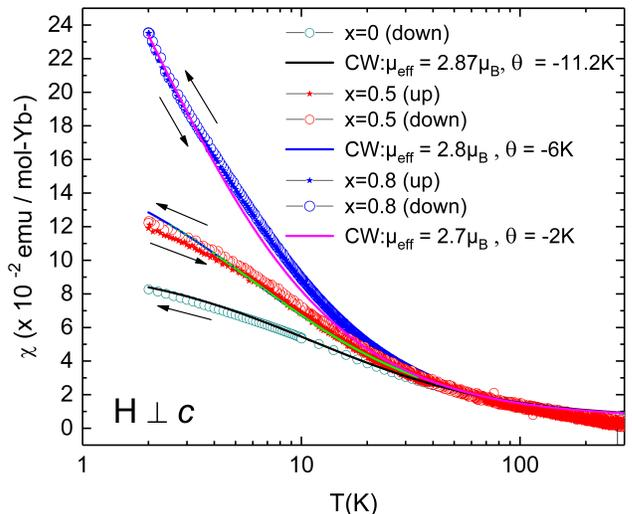
FIG. 7. Magnetic susceptibility for  $\text{NaYb}_{1-x}\text{Lu}_x\text{S}_2$  crystals with  $x = 0, 0.5$  and  $0.8$  for fields applied perpendicular to the crystallographic  $c$  direction. The solid lines represent a Curie-Weiss (CW) fit to the data below 80 K. Measurements for  $x = 0.5$  and  $0.8$  are performed in zfc(up)/fc(down) mode.
