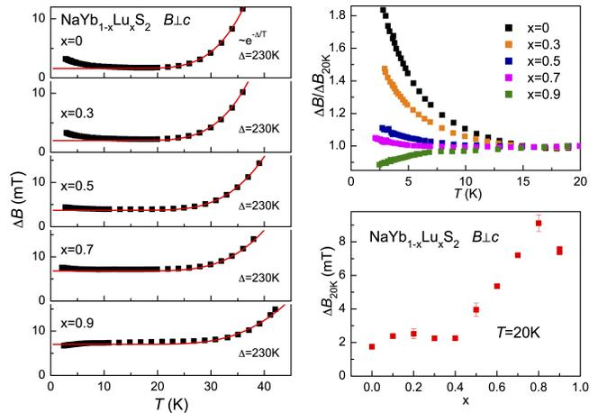
FIG. 5. Temperature- and  $x$ -dependence of the ESR linewidth  $\Delta B$  of  $\text{NaYb}_{1-x}\text{Lu}_x\text{S}_2$  single crystals. Left frame: Towards higher temperatures the solid lines indicate a relaxation via the first excited CEF level of  $\text{Yb}^{3+}$  at  $\Delta$  K. Right upper frame: Low-temperature behavior of  $\Delta B$  normalized by its value at  $T = 20$  K. Right lower frame:  $x$ -dependence of the linewidth at  $T = 20$  K.
