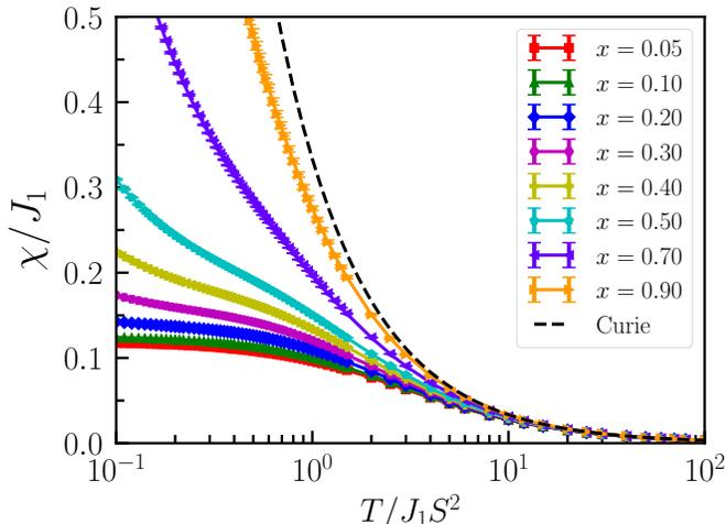
FIG. 8. Simulation results for the magnetic susceptibility per spin,  $\chi(T)/N_s$ , of the classical Heisenberg model (3) with  $J_2/J_1 = 0.12$  for different concentrations  $x$  of magnetic vacancies. The simulations were performed for  $L = 30$ ; finite-size effects are minimal for the temperatures shown.
