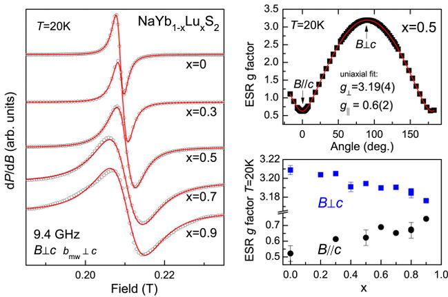
FIG. 4. Left frame: Typical X-band ESR spectra at  $T = 20$  K of  $\text{Yb}^{3+}$  for selected  $x$  in  $\text{NaYb}_{1-x}\text{Lu}_x\text{S}_2$  single crystals and for indicated field orientations. Solid lines indicate single Lorentzian line shapes. Upper right frame: ESR  $g$  factor dependence for  $x = 0.5$ , depending the field orientation with respect to the crystalline  $c$  axis. Lower right frame: Yb amount dependence of the  $g$  factor anisotropy for  $T = 20$  K.
