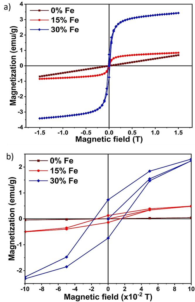
**Figure 3.** Room temperature VSM hysteresis curve of Fe-15 and Fe-30 NYF, compared with the pristine NYF sample is shown in the figure. Fig.(b) shows the enlarged view of the curve from which the magnetic remanence and coercivity are calculated.
