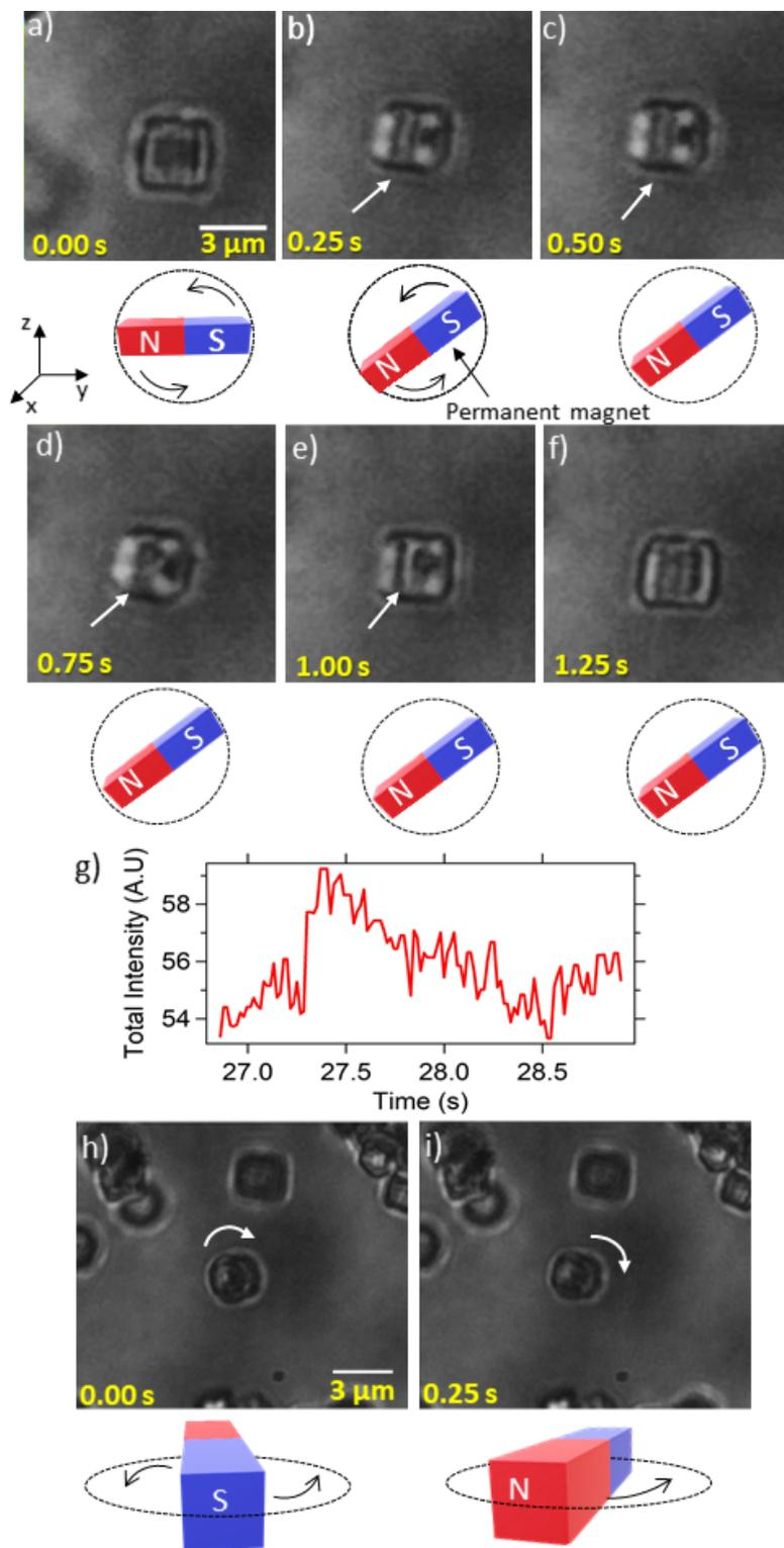
**Figure 8.** Figures (a-f) show the pitch rotational motion of an optically trapped, Fe-15 NYF upconverting particle under the influence of an external magnetic field. Fig (g) represents the corresponding time series of rotation, where the total intensity inside a rectangular region located at the tip of the arrow in figure (b) has been considered. In figures (h-i), we also show the yaw rotations of the particle under the influence of same external magnetic field.
