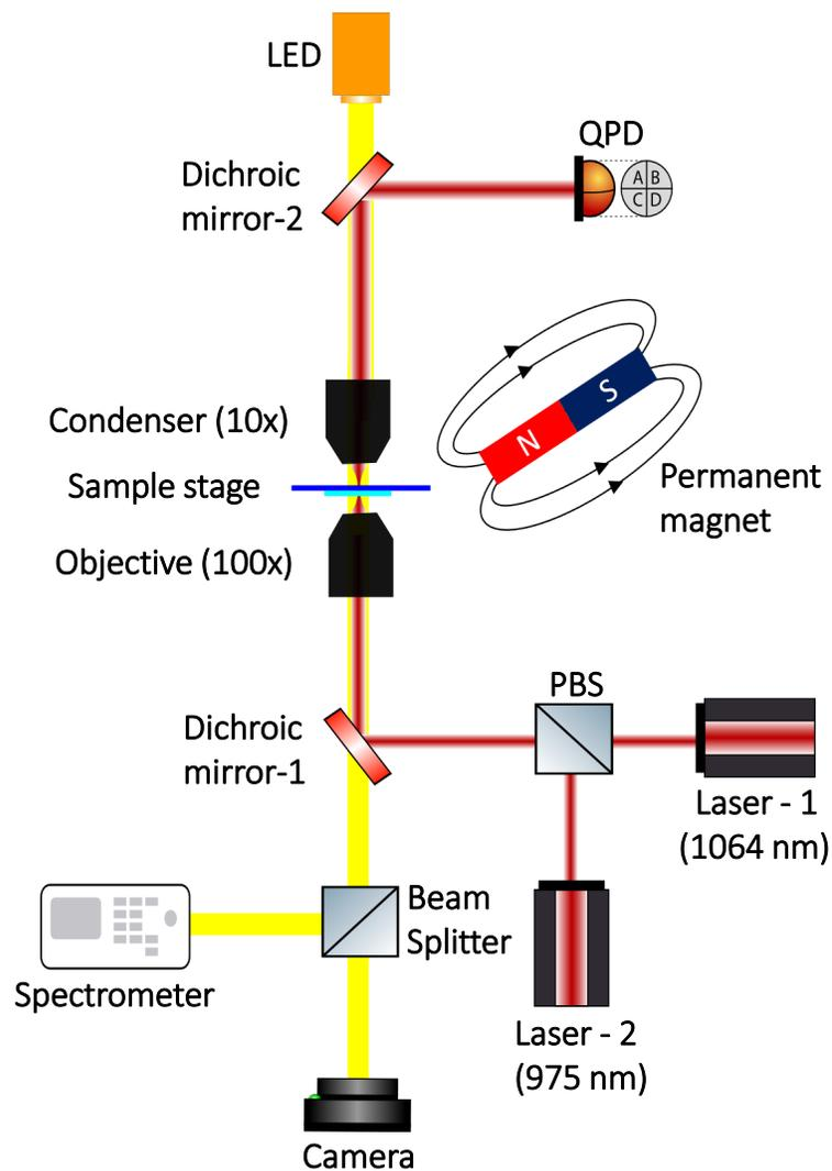
**Figure 6.** This figure represents the schematic diagram of the experiment. The entire setup consists of a single beam optical tweezers configured as an inverted microscope and its detection units. The optical trap is created near the focus of the 100x, 1.3 N.A objective and the entire sample chamber is illuminated by an LED through a dichroic mirror as shown in the figure.
