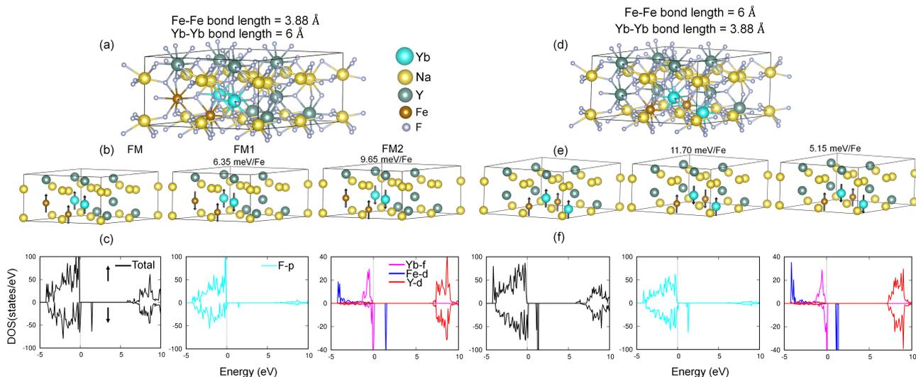
**Figure 4.** Top panel: Crystal structures of  $\text{NaY}_2\text{Yb}_1\text{Fe}_1\text{F}_4$  with Fe-Fe and Yb-Yb bond lengths being 3.88 Å, 6 Å and vice versa. Middle panel: The designed magnetic configurations: FM, FM1 and FM2. The energetics are shown with respect to the stable FM state. Bottom panel: Spin and atom resolved total density of states of most stable FM configuration.
