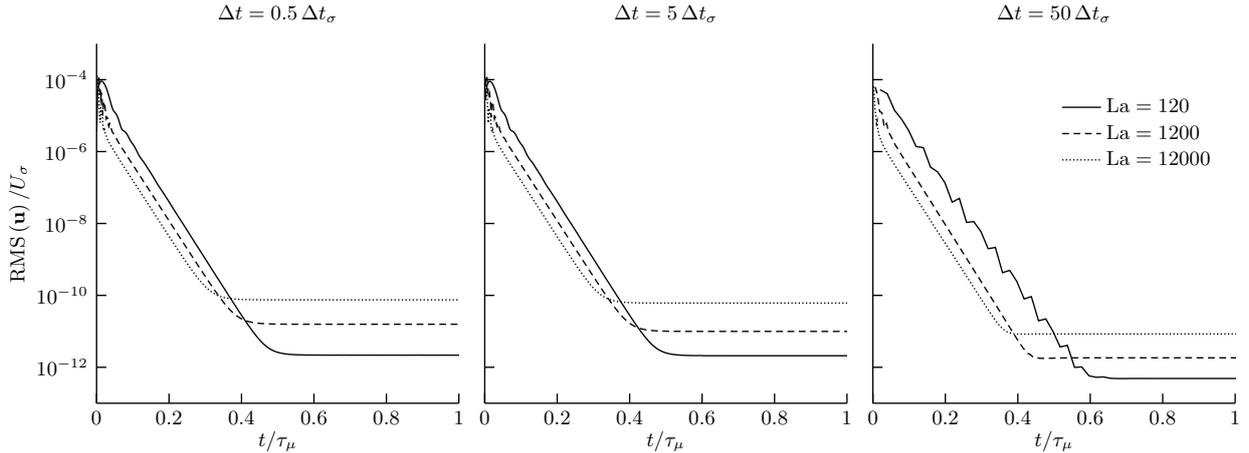
Figure 2: Evolution of the root-mean-square (RMS) of the flow velocity  $\mathbf{u}$  of the two-dimensional Laplace equilibrium with Laplace number  $La \in \{120, 1200, 12000\}$ , for different time-steps  $\Delta t$ , normalised by the capillary velocity  $U_\sigma = \sqrt{\sigma/(\rho D)}$  and the viscous timescale  $\tau_\mu = \rho D^2/\mu$ .  $\Delta t_\sigma$  refers to the capillary time-step constraint given in Eq. (3).
