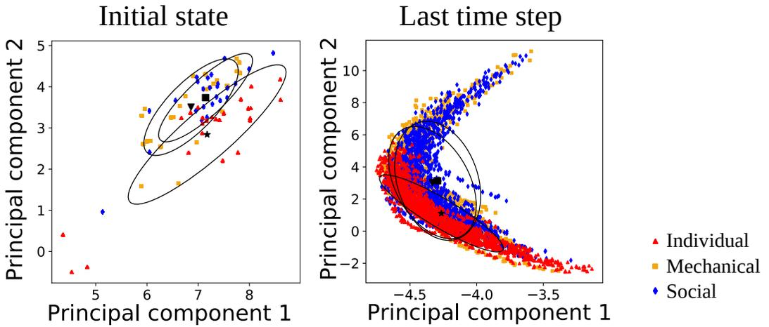
**FIGURE 7** The first two principal components of the network activation traces of one example network (capturing 83% of the variance), at the first time step (left) and at the last time step (right). The black symbols show the mean, ellipses the covariances of the points of the corresponding experimental conditions.
