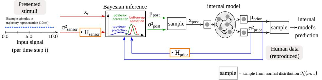
**FIGURE 1** An overview of the computational model used in the present paper: a recurrent neural network serves as the internal model that learns to predict future time steps of a one-dimensional trajectory whose length represents the length of the stimuli.
