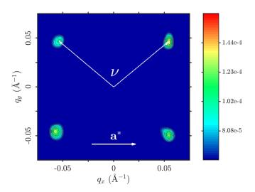
FIG. 1. A vortex lattice diffraction pattern at 23 T and 3 K. The opening angle,  $\nu$ , is used to describe the structure of the vortex lattice. The plotted signal is a measure of the counts per pixel summed along  $q_z$  divided by the product of the incident beam intensity and the square of the neutron wavelength.
