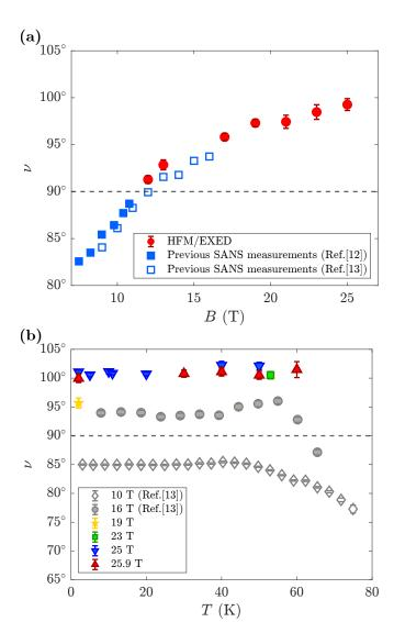
FIG. 2. (a) The evolution of the vortex lattice structure with magnetic field at 3 K. The circular points are from this study while the filled square points are from a previous study [12] up to 11 T, and the open squares are included from ref. [13]. (b) Variation of the opening angle with temperature at 25, 25.9 T with two single points at 19 T and 23 T. The diamond and circular points are from a previous study [13] and are provided for reference.
