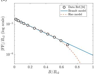
FIG. 5. Theoretical form factors versus field from numerical solution of the Eilenberger equations (points), the Hao-Clem variational solution of the GL equations (dashed line) and London model with exponential cut-off or Brandt model (solid line) versus field. Theoretical form factors calculated (a) for  $T=0.5T_{\rm c}$  using results from [23] and (b) for  $T=0.1T_{\rm c}$  using results from [24].
