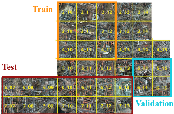
Fig. 5: The urban ISPRS Potsdam orthomosaic [1]. We simulate images and labels with a square footprint, downwards-facing camera, and GSD of 15 cm/px to generate training (orange), validation (blue), and testing (red) data from disjoint areas.
