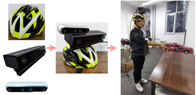
Figure 2. Data capturing system. we build up a simple head-mounted data capturing suite consists of a bicycle helmet, a Kinect v2 RGB-D sensor, and an Intel RealSense D455 RGB-D sensor.
