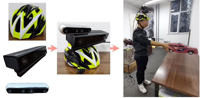
Figure 2. Data capturing system. we build up a simple head-mounted data capturing suite consists of a bicycle helmet, a Kinect v2 RGB-D sensor, and an Intel RealSense D455 RGB-D sensor.
