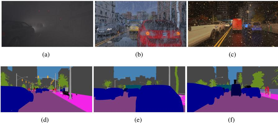
Figure 3: **Illustration of semantic segmentation images of MUAD dataset.** The first row is composed of the original images of the **high adv. set**. The second row is their corresponding ground truth.
