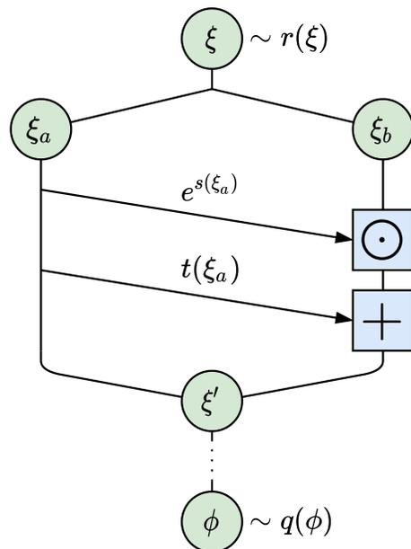
FIG. 1. Illustration of the affine coupling layer defined in [Equation \(11\)](#). The blue boxes depict element-wise operations.
