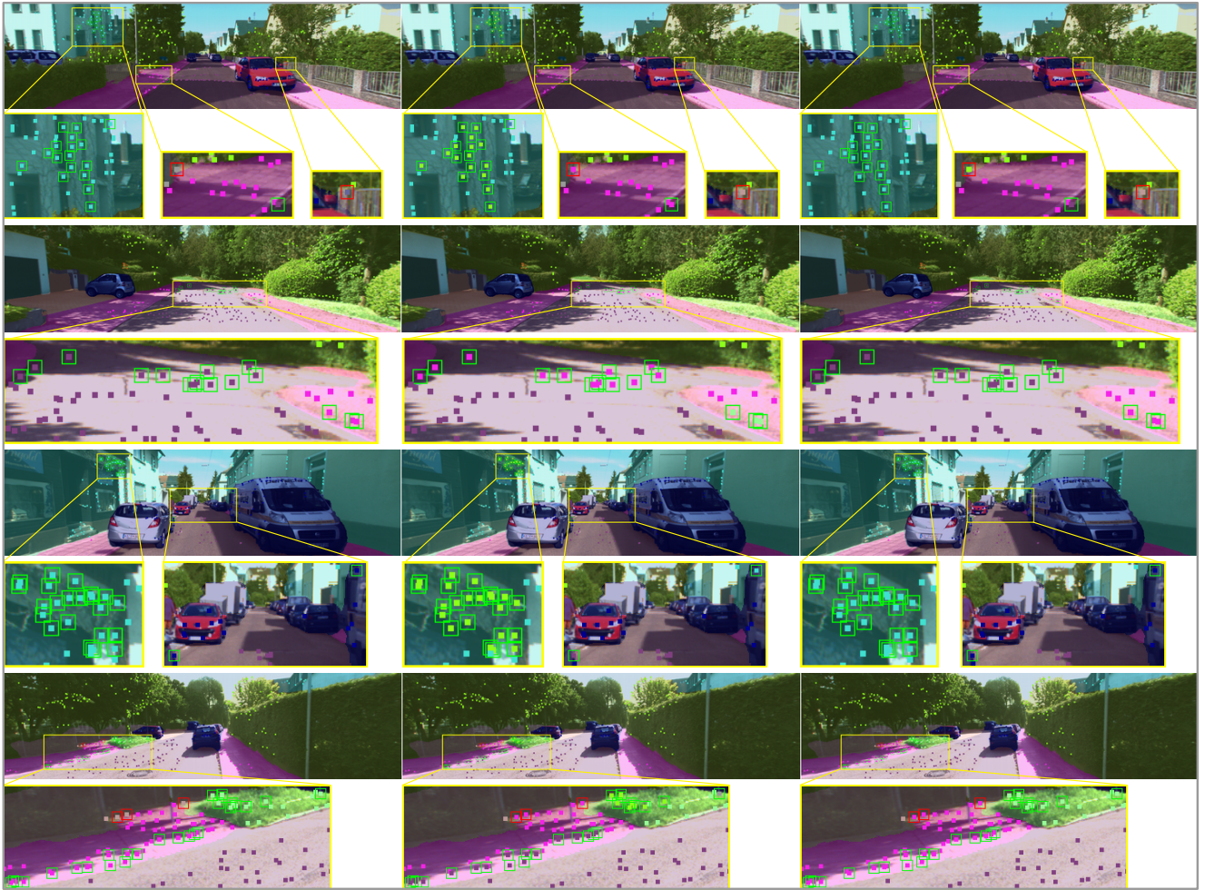
Fig. 6: Semantic point labels generated by our approach. The sparse points hosted in a keyframe are overlaid with the 2D ground truth labels and the image from KITTI-360. This is only a subset of all points in the optimization window. Two rows represent one example, where the first and second row shows the prediction results in full images and the zoom-in windows, respectively. Columns show ( left ) sparse ground truth labels, ( center ) labels predicted by the baseline model, ( right ) labels estimated by TCL, respectively. Points which are wrongly predicted by the baseline but corrected by the TCL are highlighted with green boxes. Points not corrected by the TCL are highlighted with red boxes.
