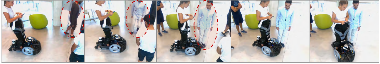
(a) Snapshot of the experiment where an adversarial pedestrian intentionally collides with the robot while a driver sets the desired velocity.
