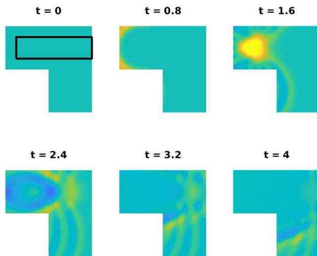
Figure 4: Waves focusing at a point in  $\Omega$ . In the section of the L-shaped domain indicated by a rectangle in the first image the wave speed is twice as fast as in the remainder of the domain.
