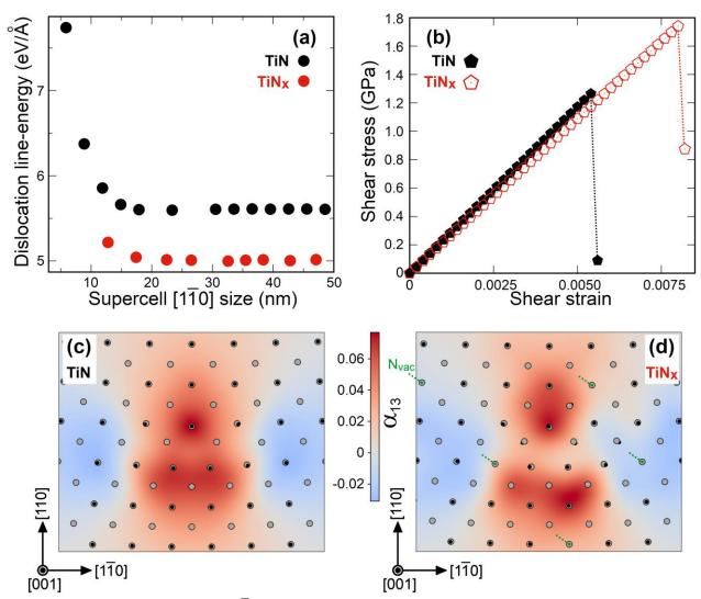
Fig. 4. MEAM results for  $\{110\}\langle 1\bar{1}0\rangle$  edge-dislocations. Qualitative comparisons of line-energies (a) and Peierls stresses  $\tau_P$  (b). Relaxed core structures and contour plots of the distribution of  $\alpha_{13}$  component of the Nye tensor in B1 TiN (c) and vacancy-ordered TiN<sub>x</sub> (d). Silver and black spheres represent Ti and N atoms, respectively. Green dashed arrows in (d) indicate positions of nitrogen vacancies (N<sub>vac</sub>) in the plane of view.
