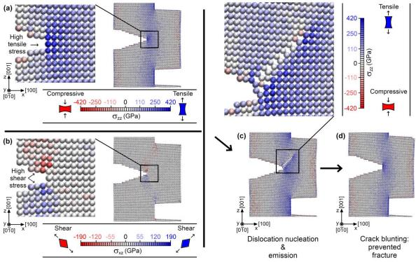
**Fig. 7**. Results of a simulation with different initial velocities than in **Fig. 6** (see **Video#4** in **SM** [20]). (a) High tensile stress combined with (b) relatively high shear stress assists (c) nucleation and emission of dislocations, which (d) blunts the crack and prevents fracture. In (a) and (b), the simulation box is strained by 5%.
