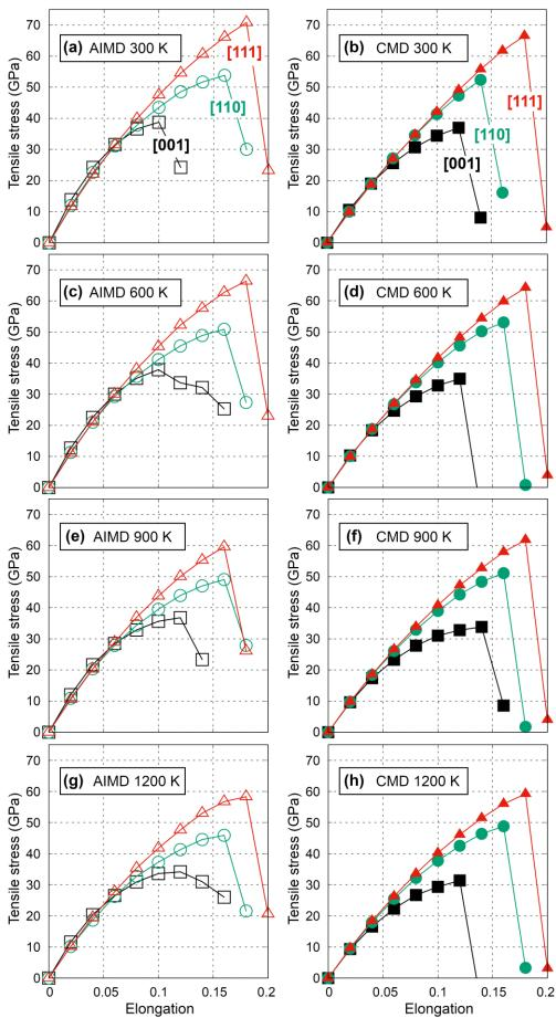
**Fig. 3**. AIMD **(a,c,e,g)** vs CMD **(b,d,f,h)** results for tensile deformation (Cauchy stress/strain) of stoichiometric defect-free TiN as a function of temperature. All curves end with the fracture point. AIMD stress strain data at room temperature presented in panel **(a)** are taken from Ref. [16].
