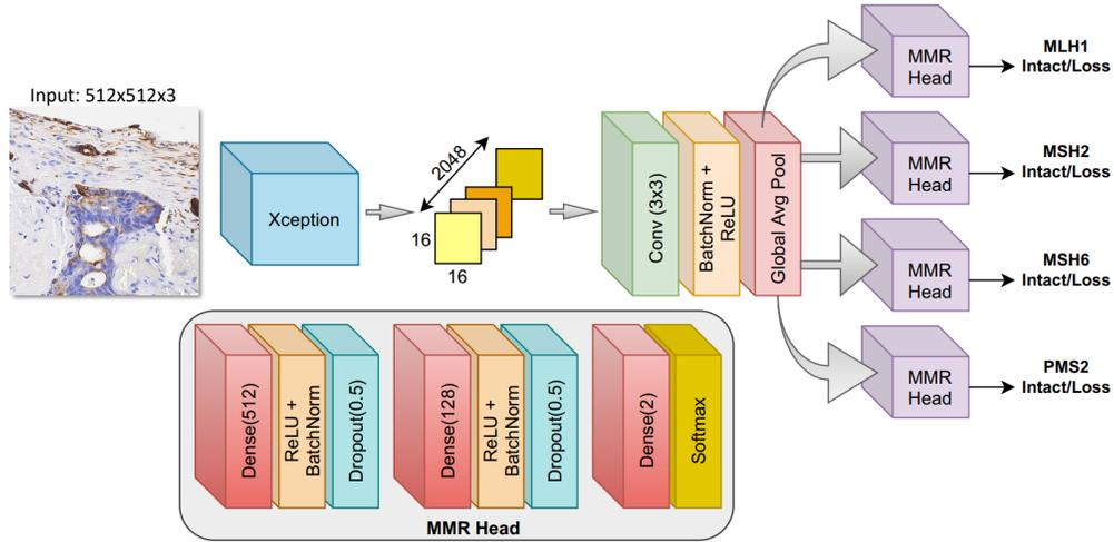
Supplementary Figure 4: The proposed CNN architecture for MMR prediction.
