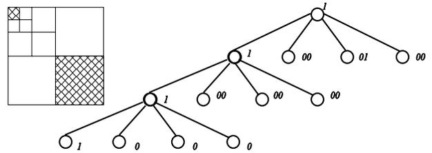
fig. 4 modified quadtree for inter/intraframe predictor. Last level and second bit of terminal nodes codifies the inter/intra frame decision. Dashed squares are intraframe coded zones.
