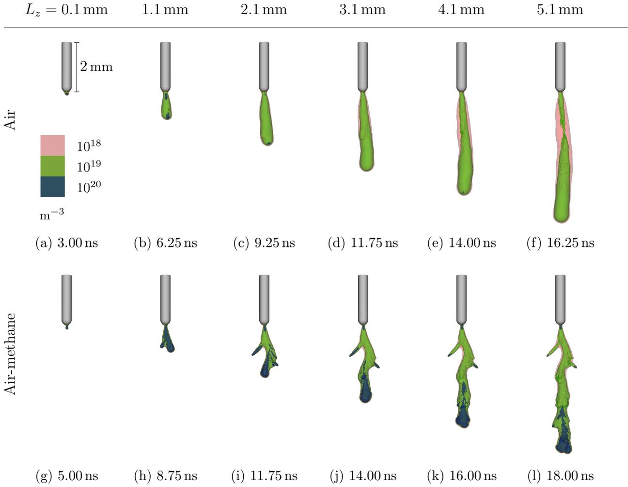
Figure 5: Evolution of the electron density for positive streamers as a function of streamer length. Streamers propagate in a background field of  $E_0 = 12.5 \text{ kV/cm}$  in air (top) and air-methane (bottom). The corresponding simulated times are supplied in the sub-caption. Visualization is performed with three partially-transparent contour surfaces. We observe that shape of the air streamer is smooth whereas the air-methane streamer is more erratic.
