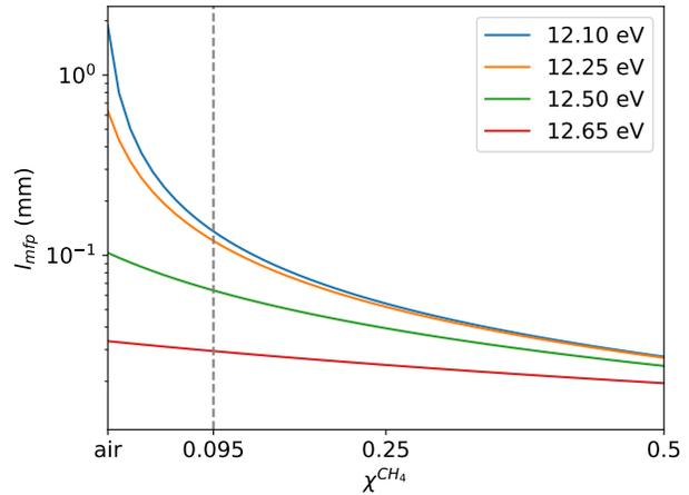
Figure 2: The photon mean free path as a function of the  $\text{CH}_4$  fraction  $\chi^{\text{CH}_4}$  in air-methane mixtures for various photon energies. Stoichiometric conditions are denoted by the dashed grey line. Adding methane shortens the photon mean free path.
