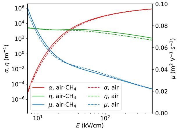
Figure 1: The transport and reaction coefficients for air and stoichiometric air-methane at 1 bar and 300 K. The axis for the mobility  $\mu$  is linear, whereas the axis for ionization and attachment coefficients  $\alpha$  and  $\eta$ , respectively, is logarithmic. We conclude that a gas fraction of 9.5%  $\text{CH}_4$  introduces only minor changes to these coefficients.
