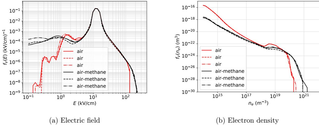
Figure 8: The volume distribution  $f_V(E)$  of the electric field strength and  $f_V(n_e)$  of the electron density. We have shown three air streamers and three air-methane streamers at a length of 5.1 mm under conditions corresponding to figure 5. Air-methane streamers exhibit stronger electric field enhancement and higher electron densities.
