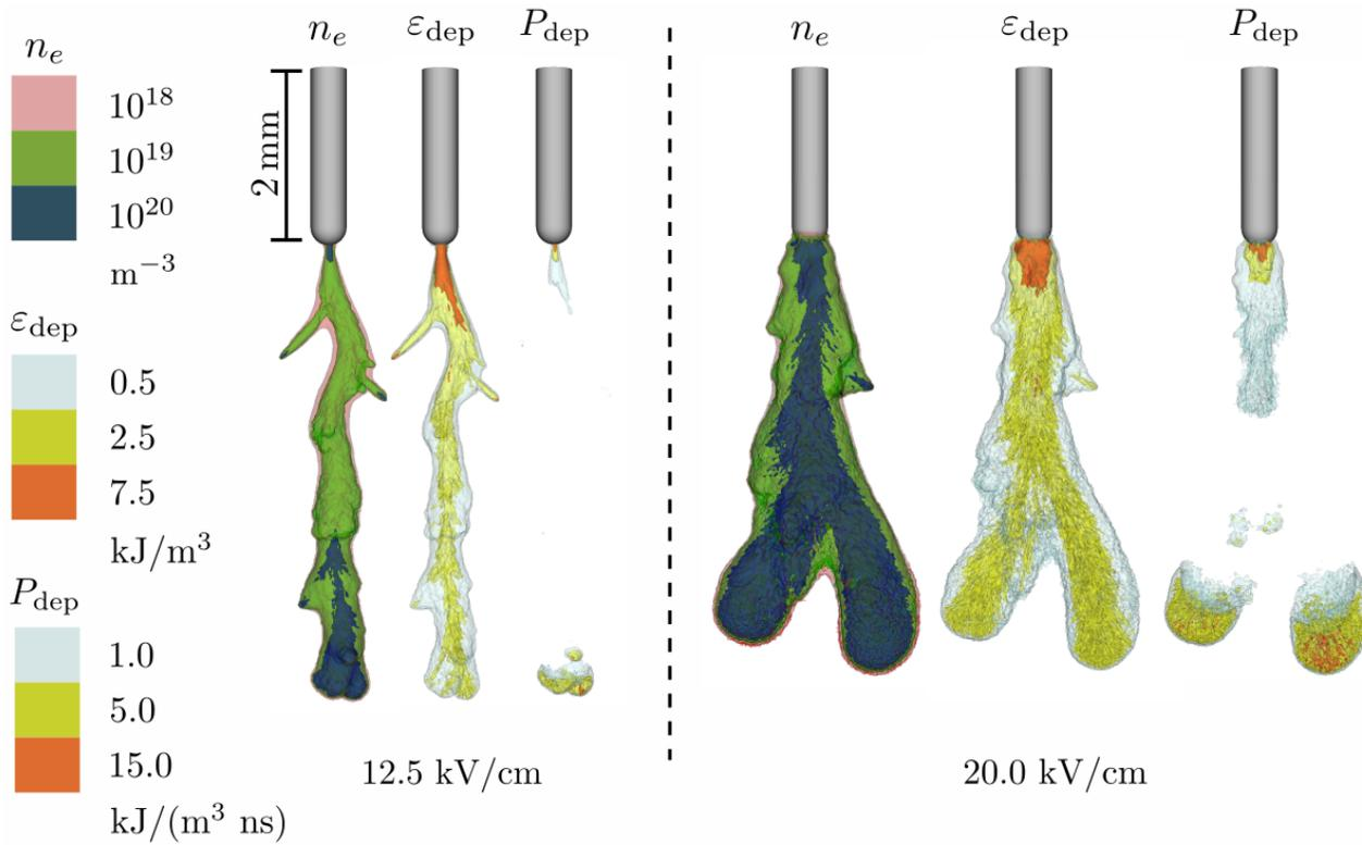
Figure 10: Contour surfaces of the electron density, the deposited energy density and the power density deposition within 0.25 ns. We show air-methane streamers with a length of  $L_z = 4.8$  mm in two background fields. Due to a higher velocity in higher electric fields, the contribution of the ionization front to  $P_{\text{dep}}$  appears more smeared out.
