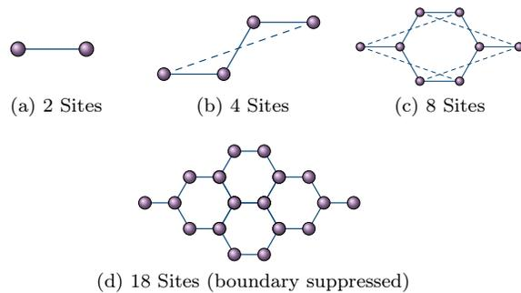
Figure 1. Graphical representation of the arrangement of ions considered in the numerical investigation. Each node corresponds to an ion while each edge indicates an allowed particle/hole hopping. The dashed lines represent the periodic boundary.
