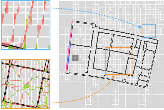
Fig. 1. Approximate Nearest Neighbor Fields (ANNF) with at most d = 5 layers in depth. Every quadratic subfield stores two nearest elements from the floor plan. For example, the highlighted subfield marked with a cross stores a blue line segment as its nearest neighbor and a pink line segment as its second nearest neighbor. The data structure can be constructed up-front, and can be used as a look-up table with \mathcal{O}(d) complexity. On the left, we show a performance validation as two zoom-in figures. The orange dot indicates a tested position that has the second nearest element from the ANNF as its closest element. The green dot indicates a location where the ANNF search did not include the ground truth closest element. An interactive demo can be found at https://mpl-annf.github.io/
