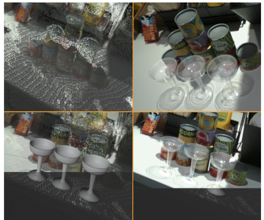
Fig. 9: The labelling on transparent champagne cups. When there is no reliable depth (top-left), ProgressLabeller enables checking the pose validity by re-projection object models (bottom-left) to RGB images from different views (top-right and bottom-right).
