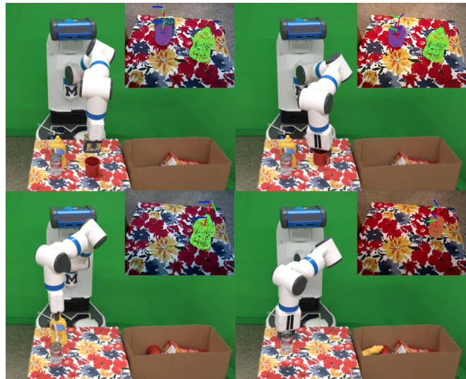
Fig. 7: The Fetch robot is grasping objects on tabletop based on estimated poses. The pose estimates are shown as projected point clouds and coordinate frames in top-right smaller images. The higher and lower frames correspond to pre-grasp and grasp poses.
