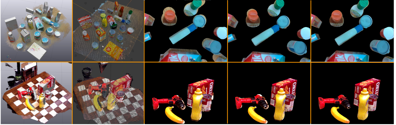
Fig. 4: From left to right, we show the 3D labeler view of LabelFusion, ProgressLabeller and cropped RGB image with masks from LabelFusion, ground truth and ProgressLabeller. The top and bottom row show a sample from HOPE and YCB dataset respectively. We find even ground truth pose labels have easily observable errors, shown as the spacing between black masks and object boundaries.
