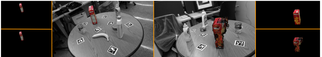
Fig. 8: Comparison of best (left) and worst (right) validation pose renderings from the NSVF model. The smaller images with black background on top corners are the ground truth masks, and those on bottom corners are rendered output from NSVF, and the middle larger images are the renderings imposed onto the original captured image in greyscale. The best image (left) had an average pixelwise L2 error of 0.0067, and the worst (right) had an average pixelwise L2 error of 0.1867.
