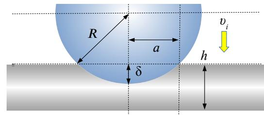
**Fig. 4** (Color online) The geometrical parameters involved in the collision between a viscoelastic board, with a thickness of  $h$ , and a solid sphere, with its radius  $R$  in the impact-velocity  $v_i$ . The deformation  $\delta$  and diameter of contact  $a$  are generated by the collision with the viscoelastic board.
