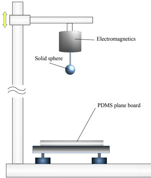
**Fig. 2** (Color online) Sketch of experimental setup. The solid ball is suspended by an electromagnet. The velocity of impact is adjusted by changing the height of the part suspending the sphere. The sphere ( $R = 3.0, 4.0, 5.0, 6.0, 7.0$  and  $8.0$  mm,  $\rho = 7800 \text{ kg} \cdot \text{m}^{-3}$ ) is dropped onto the PDMS plane board ( $\phi = 1, h = 6.4$  mm) by turning off the electromagnet.
