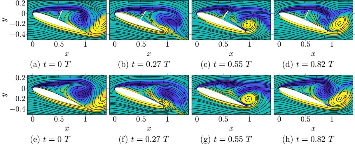
FIG. 2: Vorticity contours depicting vortex shedding from the leading and trailing edges of the airfoil for a representative case of  $k_\beta = 0.001$ ,  $m_\beta = 1.875$  and 50% location (top row) and the flap-less baseline airfoil case (bottom row) at four time instants in a lift cycle.
