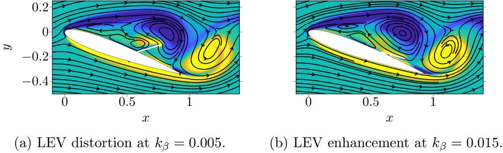
FIG. 20: Demonstration of LEV deformation as it advects above the flap at  $t/T = 0.82$  for  $m_\beta = 1.875$  and 60% location via vorticity contours.
