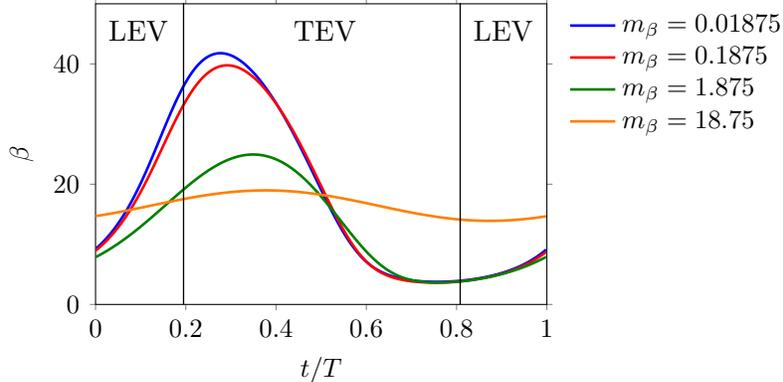
FIG. 23: Flap deflection in one time period of the lift cycle for 60% location and  $k_\beta = 0.015$ . The time period is divided into two portions dominated by the LEV and TEV where the time instants of demarcation are  $t/T \approx 0.2$  and  $t/T \approx 0.8$ .
