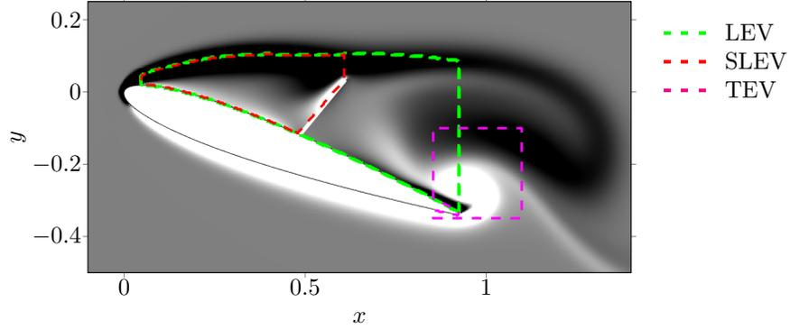
FIG. 31: Demonstration of areas of integration for quantifying LEV, SLEV and TEV strengths.
