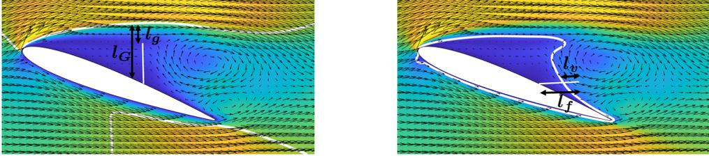
(a) Gap ratio in flap-shear interaction regime (b) Flap ratio in flap-vortex interaction regime
