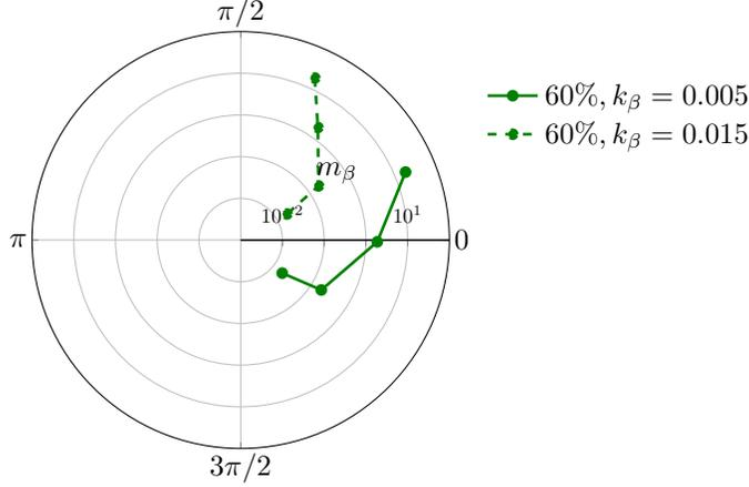
FIG. 24: Phase difference of flap oscillations  $v/s$  mass ratio (along the radial axis) for various stiffness at 60% location.
