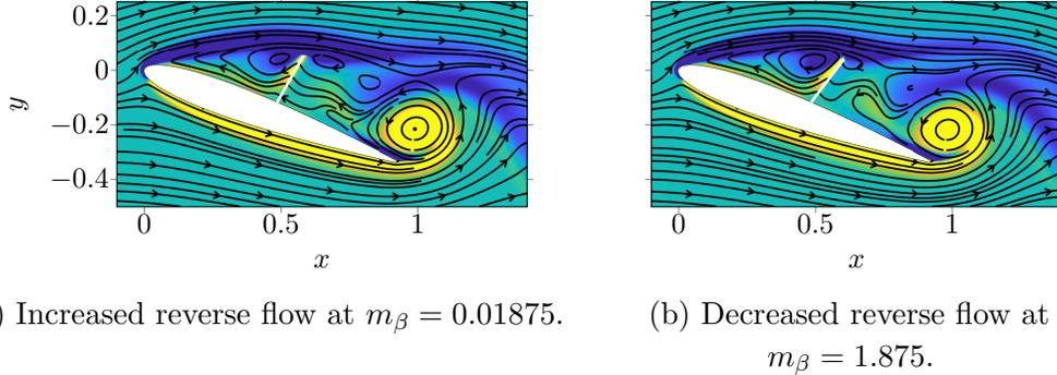
FIG. 12: Demonstration of propagation of TEV-induced reverse flow facilitated by the upstream oscillation of the flap via vorticity contours and superimposed streamlines at  $t/T = 0.55$  for  $k_\beta = 0.0015$  and 50% location.
