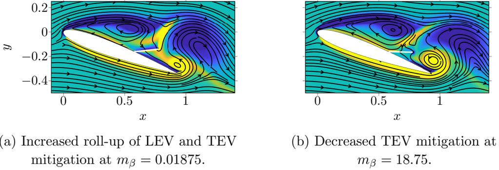
FIG. 25: Demonstration of the mitigation of TEV and roll-up enhancement of LEV facilitated by the downward-oscillating flap via vorticity contours with superimposed streamlines at  $t/T = 0.45$  for  $k_\beta = 0.015$  and 60% location.
