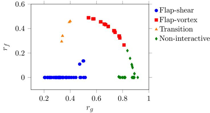
FIG. 30: Clusters determined by the k-means algorithm with gap ratio,  $r_g$  and flap ratio,  $r_f$  as the inputs. The data points include all the cases of mass ratio, stiffness and hinge location considered in the parametric study.
