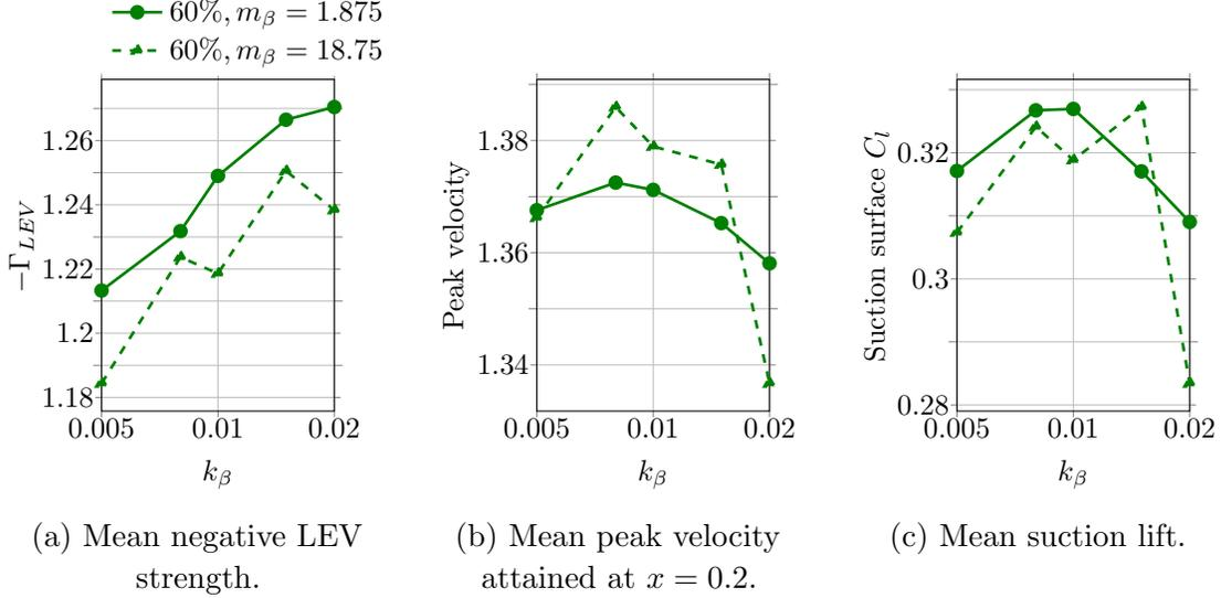
FIG. 21: Plots of various physical quantities characteristic of static behavior in the flap-vortex regime averaged over a time period for 60% location,  $m_\beta > 1$  and varying stiffness.
