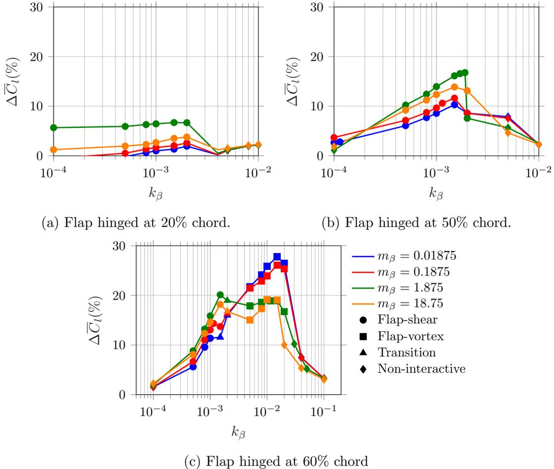
FIG. 4: Performance plots showing percentage change in mean lift for the various cases of mass ratio, stiffness and hinge location. The marker symbols denote the flow regimes identified using a flow classification algorithm described in Appendix A.
