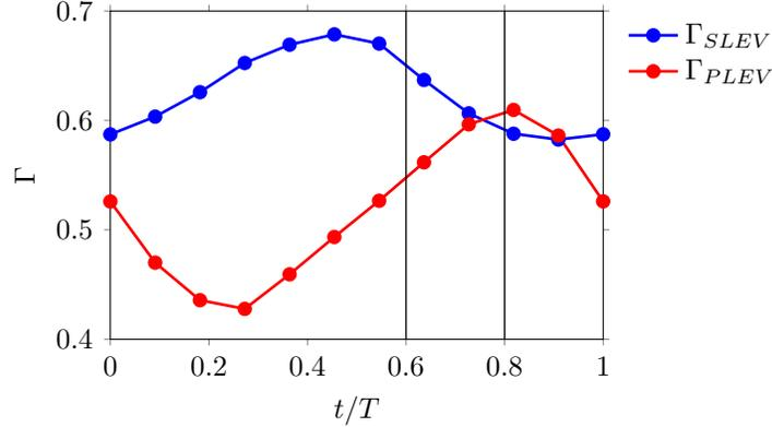
FIG. 16: Vortex circulation strengths in one time period of the lift cycle for 50% location,  $m_\beta = 1.875$  and  $k_\beta = 0.0015$ . The region between the black vertical lines,  $t/T \in [0.6, 0.8]$ , denotes the SLEV-to-PLEV transfer process.
