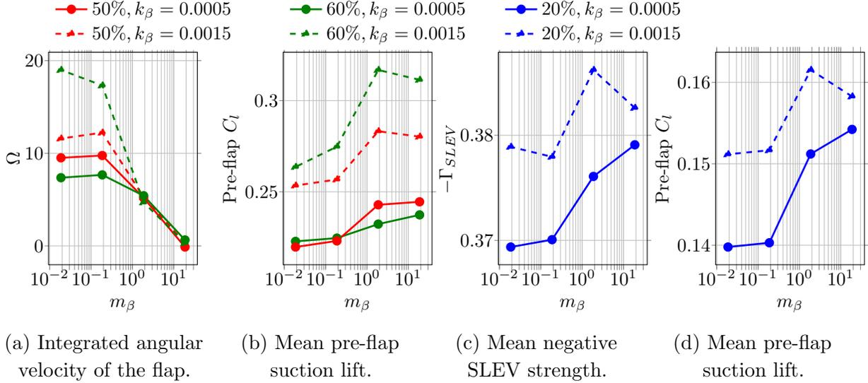
FIG. 14: Plots of various physical quantities characteristic of dynamic behavior in the flap-shear interaction regime averaged or integrated over the TEV-dominant portion of the lift cycle for different locations, mass ratios and stiffness.
