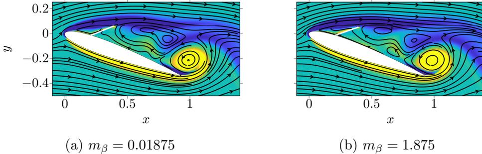
FIG. 15: Demonstration of insubstantial variations in TEV-induced reverse flow for upstream 20% flap location and  $k_\beta = 0.0015$  via vorticity contours and superimposed streamlines at  $t/T = 0.55$ .
