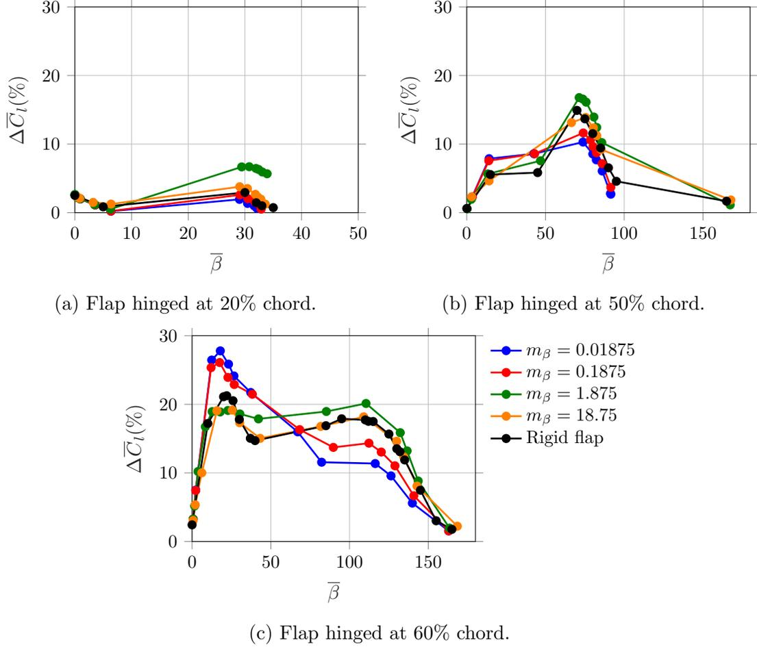
FIG. 5: Performance plots showing percentage change in mean lift for the various cases of inertia, stiffness-dependent mean flap deflection and hinge location. The rigid flap cases correspond to a stationary rigid flap affixed at various deployment angles.
