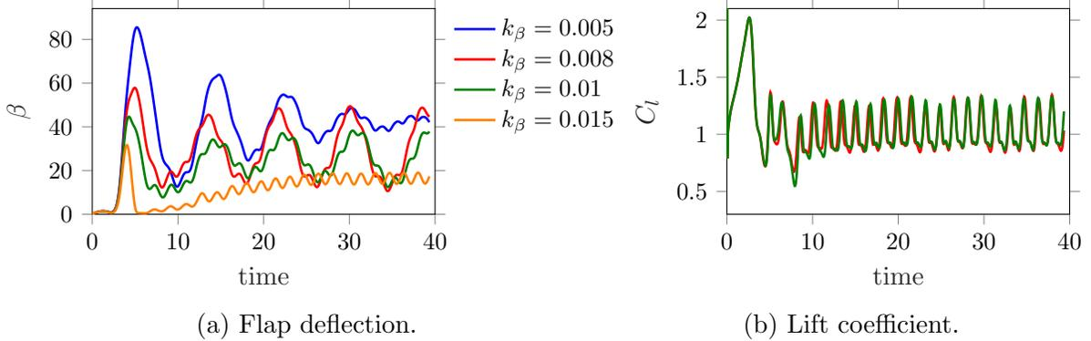
FIG. 22: Demonstration of the presence of dual frequencies in the flap deflection signal only minimally affecting the frequency of the airfoil lift signal for select stiffness values at the largest mass ratio of  $m_\beta = 18.75$  and 60% location.
