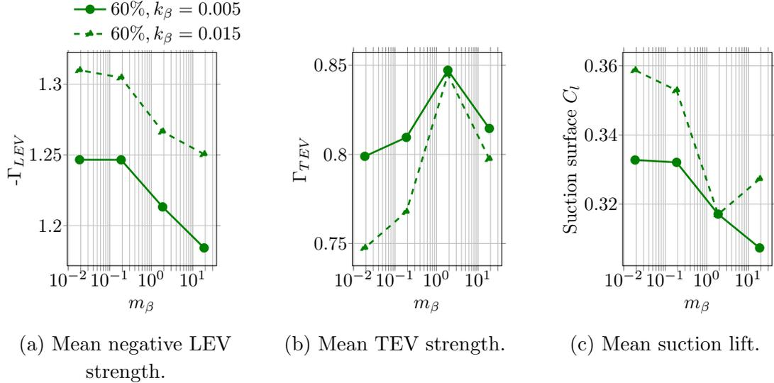
FIG. 26: Plots of various physical quantities characteristic of dynamic behavior in the flap-vortex interaction regime averaged over one time period for 60% location, and varying mass ratio and stiffness.
