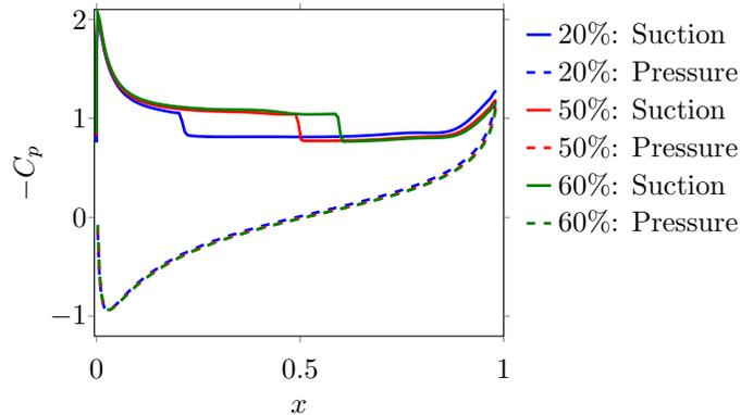
FIG. 10: Comparison of the pressure dam effect at different flap locations via mean  $C_p$  distribution for  $m_\beta = 1.875$ ,  $k_\beta = 0.0015$ .
