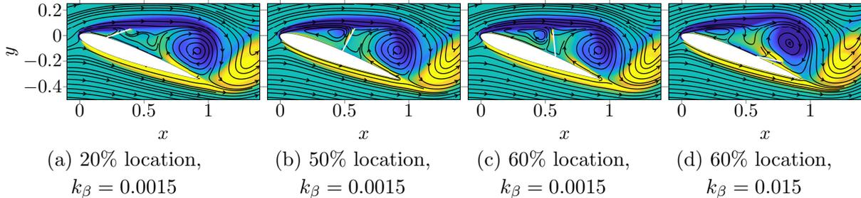
FIG. 6: Vorticity contours demonstrating flap configurations in the flap-shear (subplots (a), (b) and (c)) and flap-vortex (subplot (d)) interaction regimes. The contours are plotted at a representative time instant of  $t/T = 0$  and  $m_\beta = 1.875$ .
