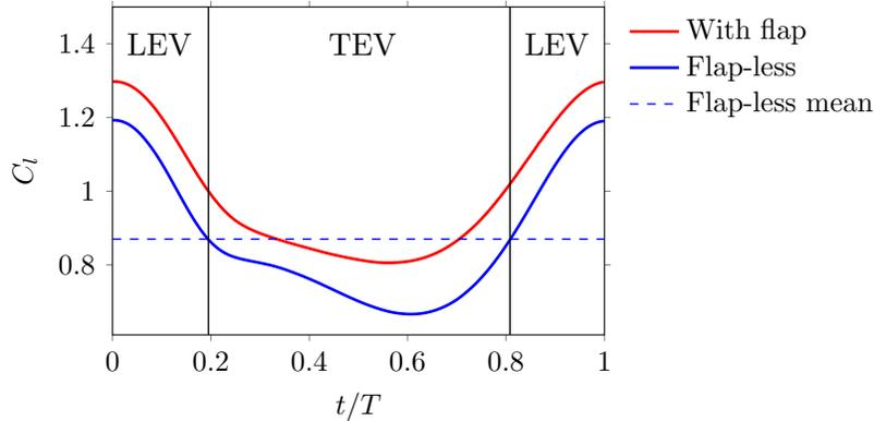
FIG. 3: Coefficient of lift in one time period of the lift cycle for the flap (50% location,  $k_\beta = 0.001$ ,  $m_\beta = 1.875$ ) and flap-less cases. The time period is divided into two portions dominated by the LEV and TEV where the time instants of demarcation are  $t/T \approx 0.2$  and  $t/T \approx 0.8$ .
