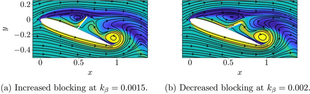
FIG. 9: Demonstration of the stiffness-dependent flap deployment angle dictating the magnitude of blocking of propagation of TEV-induced reverse flow via vorticity contours and superimposed streamlines at  $t/T = 0.55$  for  $m_\beta = 1.875$  and 50% location.
