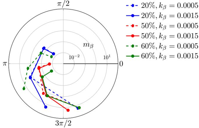
FIG. 13: Phase difference of flap oscillations  $v/s$  mass ratio (along the radial axis) for various stiffness and locations.
