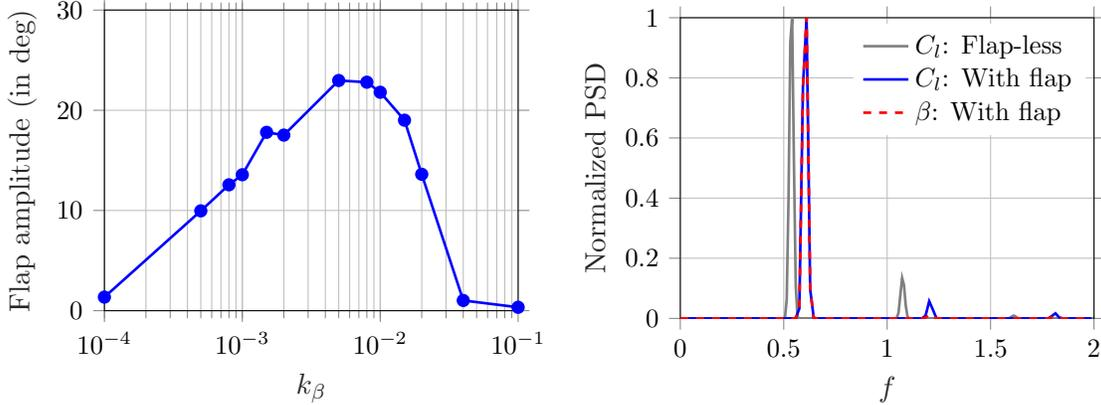
(a) Amplitude of flap oscillations for a flap hinged at 60% location and  $m_\beta = 0.01875$ . (b) Normalized power spectral density (PSD) of the lift and flap deflection signals for the flap-less case and the case of flap hinged at 60% location,  $k_\beta = 0.015$  and  $m_\beta = 0.01875$ .
