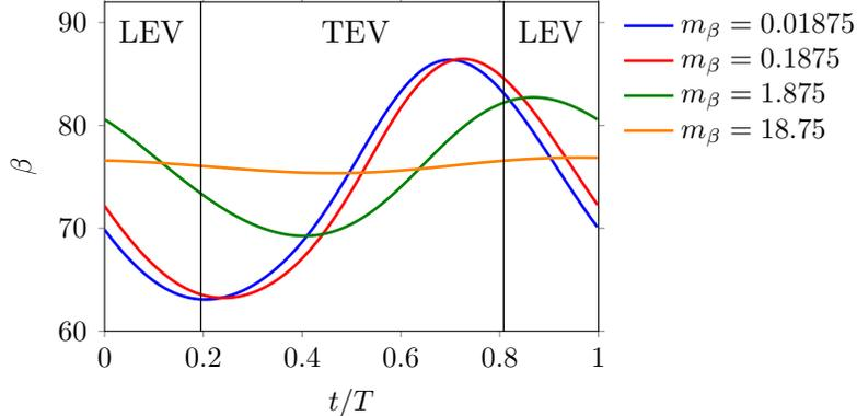
FIG. 11: Flap deflection in one time period of the lift cycle for 50% location and  $k_\beta = 0.0015$ . The time period is divided into two portions dominated by the LEV and TEV where the time instants of demarcation are  $t/T \approx 0.2$  and  $t/T \approx 0.8$ .
