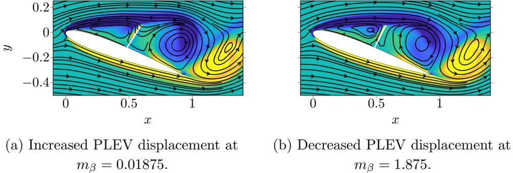
FIG. 17: Demonstration of downstream displacement of PLEV facilitated by the downward oscillation of the flap via vorticity contours and superimposed streamlines at  $t/T = 0.91$  for  $k_\beta = 0.0015$  and 50% location.
