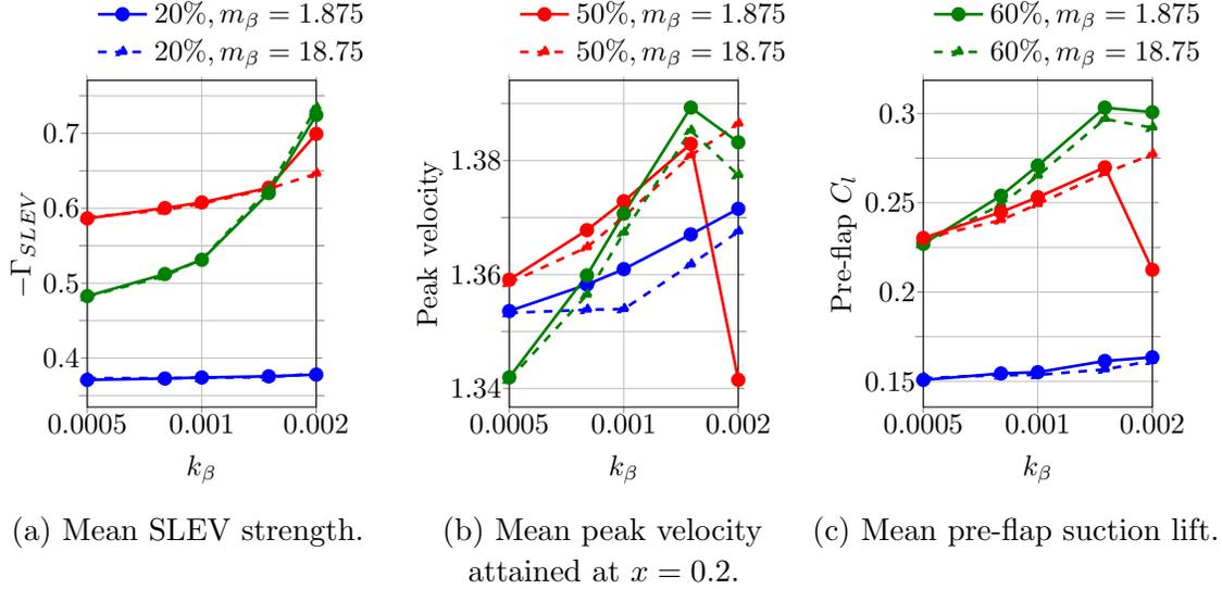
FIG. 8: Plots of various physical quantities characteristic of static behavior in the flap-shear regime averaged over a time period for  $m_\beta > 1$  cases.
