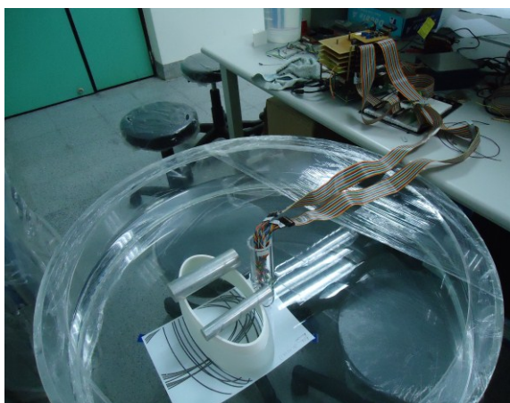
Fig 2 The experimental probe submerged in ionized water in the middle of the water tank
