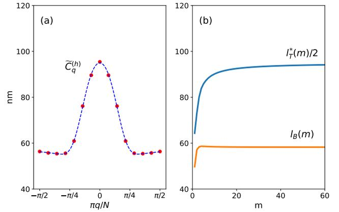
Figure 4. (a) Q-stiffnesses of the helical twist of RNA as obtained from all-atom data. (b) Length-scale-dependence of the twist (blue) and bending (orange) persistence lengths for RNA duplexes. The length-dependence of  $l_T^*(m)/2$  is derived from equation (9) using the  $q$ -stiffnesses displayed in (a).  $l_B(m)$  is acquired using equation (13) along with the attained momentum-space stiffnesses exhibited in Figure 2(b).
