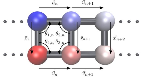
Figure 5. Schematic of the ladder model in its ground-state configuration. Intra- and inter-strand bond vectors are denoted with  $\vec{u}$ ,  $\vec{v}$  and  $\vec{x}$  respectively.
