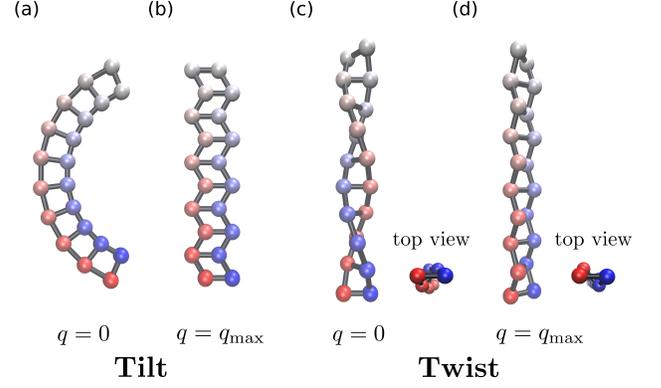
Figure 8. Ladder configurations corresponding to distinct  $q$ -modes:  $q = 0$  for (a,c) and  $q = (N-1)/2$  for (b,d). (a,b) and (c,d) represent pure tilt and twist deformations, respectively. The ladders displayed are small subsystems extracted from infinitely long ladders, such that on the scale of the figure angular modulation for (b,d) are omitted.
