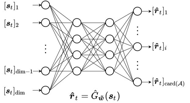
Fig. 2. The structure of the reward-prediction network  $\hat{G}_{\hat{w}}$  of the proposed DRP algorithm. The network receives a channel observation as input and outputs its predicted expected reward for each of the actions in the action space.
