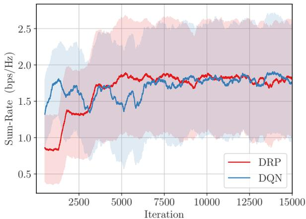
Fig. 4. Training curves of the compared DRL algorithms for the first portion of the training period. The curves are smoothed by averaging within a rolling window of 300 iterations, and the shaded areas represent the accompanying standard deviations.  $P$  is set to 40 dBm and  $N_{\text{tot}}$  to 96.
