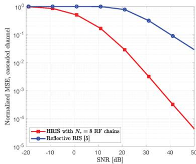
Fig. 5. Normalized MSE performance in estimating the cascaded channel via an HRIS and a purely reflective RIS versus the transmit SNR in dB.
