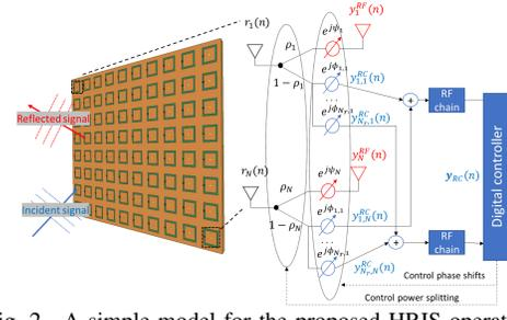
Fig. 2. A simple model for the proposed HRIS operation.
