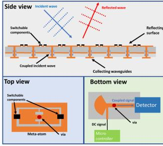
Fig. 1. Illustration of the proposed hybrid metamaterials.
