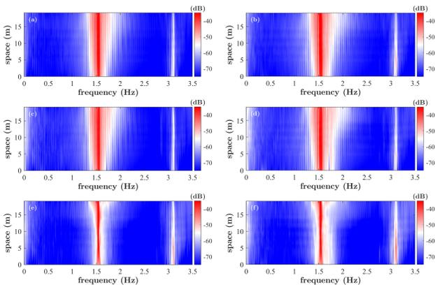
FIG. 3: Spectral evolution of the standing Peregrine breathers, reported in Fig. 2. (a) Computed for the measured surface elevation for the carrier parameters  $a = 0.01$  m and  $ak = 0.09$ . (c) Incident PB wave dynamics isolated from (a). (e) Opposing wave train as isolated from (a). (b) Computed for the measured surface elevation for the carrier wave parameters  $a = 0.01$  m and  $ak = 0.10$ . (d) Incident PB wave dynamics isolated from (b). (f) Opposing wave train as isolated from (b).
