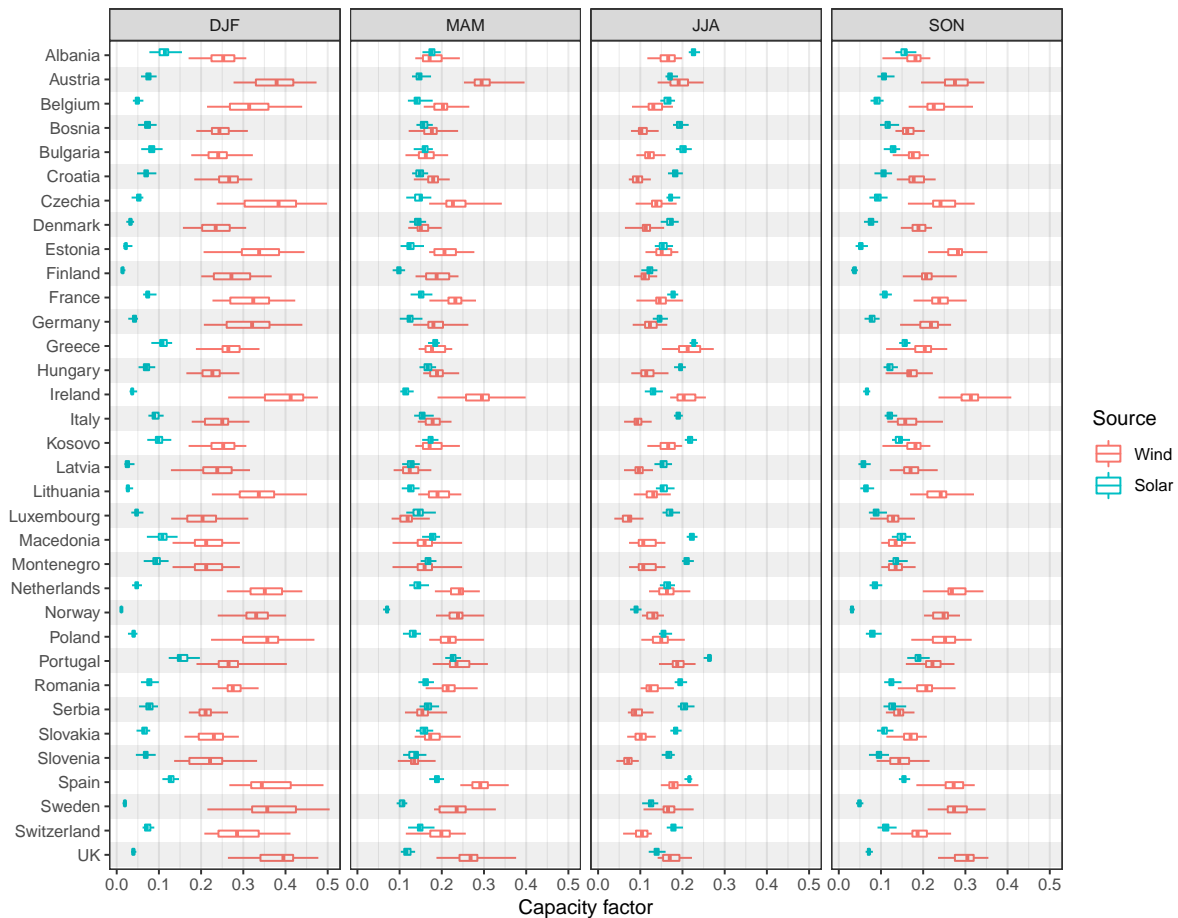
Figure 4: Interannual variability of wind (red) and solar (blue) seasonal-mean capacity factors in the 1986–2015 period for 34 European countries, according to the EMHIREs dataset. Each boxplot represents the 30 seasonal-mean values for a given season, generation type and country. The whiskers depict the range (min-max) and the boxes the three quartiles.
