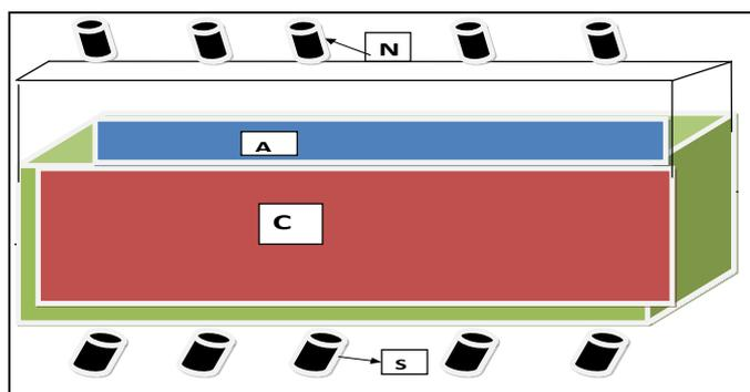
**Figure 8.** An inhomogeneous magnetic field can enhance the yield of  $H_2$ . The magnets with north poles N and south poles S must possess a bigger extension as show in the above Figure. All magnets are permanent magnets (ferro-magnets). The radiation beam passes between these plates.
