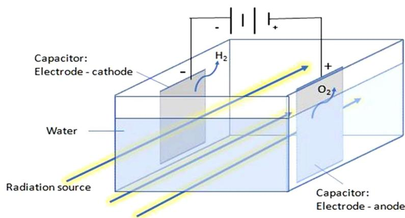
Figure 4. Basic configuration of an electrolyser using external  $\gamma$ -rays and two capacitors for cathode and anode
