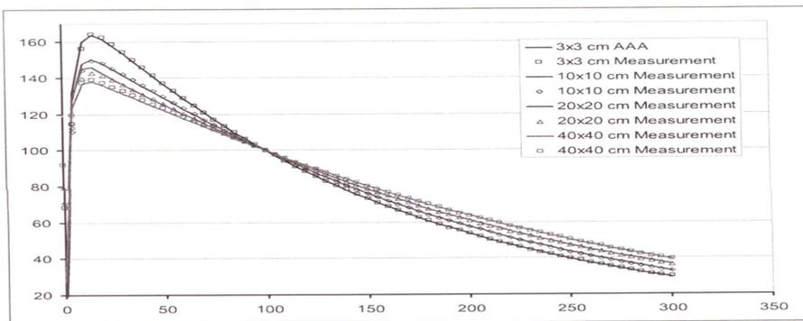
**Figure 6.** Depth dose curves of 6 MV 'bremsstrahlung' of a Linac (Ulmer, et al., 2005).
