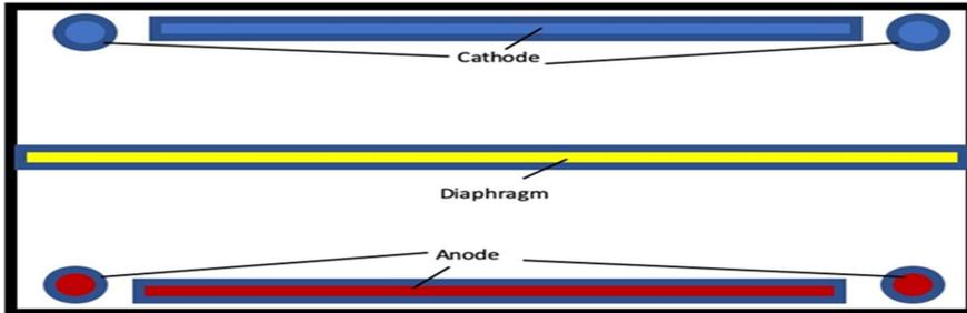
**Figure 5.** Top view on electrolyzer with the capacitor plates and additional electrodes. The use of a diaphragm is optional and serves for separation of H<sub>2</sub> and O<sub>2</sub> gases to avoid the formation of explosive gas mixtures.
