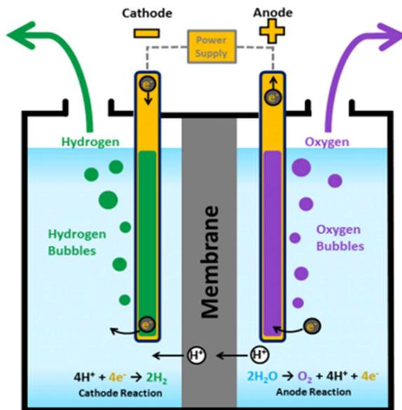
Figure 1. Schematic representation of the water electrolysis – the complete apparatus is referred to as electrolyzer (see e.g., Review in DOE Hydrogen Program, 2020, Kato, 2003, Walter, 2010).
