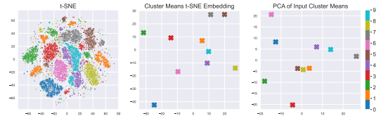
Figure 1: Left: MNIST t-SNE (perp : 30) embeddings initialized with i.i.d \mathcal{N}(0, 1) coordinates. Middle: using these t-SNE embeddings, mean coordinates for each digit are represented. Right: we compute a matrix of mean input coordinates for each of the 10 digits and embed it using PCA. For t-SNE embeddings, the positions of clusters vary across different runs and don't visually match the PCA embeddings of input mean vectors (right plot).
