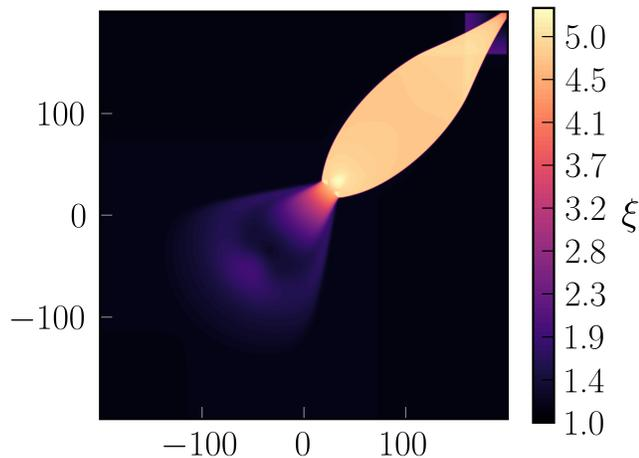
FIG. 5. Solution for the log of the energy density,  $\xi$ , for the 2D oblique shockwave initial data (53) at  $t \sim 220$  for  $\eta_0 = 0.2$ . Note that the solution is non-oscillatory, even though there is an order unity jump in  $\xi$  (corresponding to a jump of  $\sim 50$  in  $\epsilon$ ) which is not aligned with the numerical grid.
