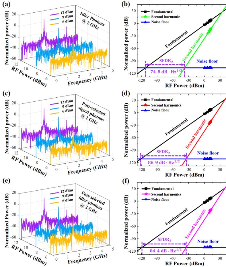
Fig. 4. The DFT spectra of (a) the directly measured idler photon waveforms, (c) the post-selected signal photon waveforms, and (e) the post-selected idler photon waveforms. Different
