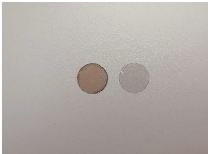
Figure S4 Photography of muscovite mica substrate: a) Purchased mica substrate (Electron Microscopy Science) with thickness of 0.15-0.21 mm and b) scotch tape exfoliated mica substrate for IR-AFM experimental set-up.
