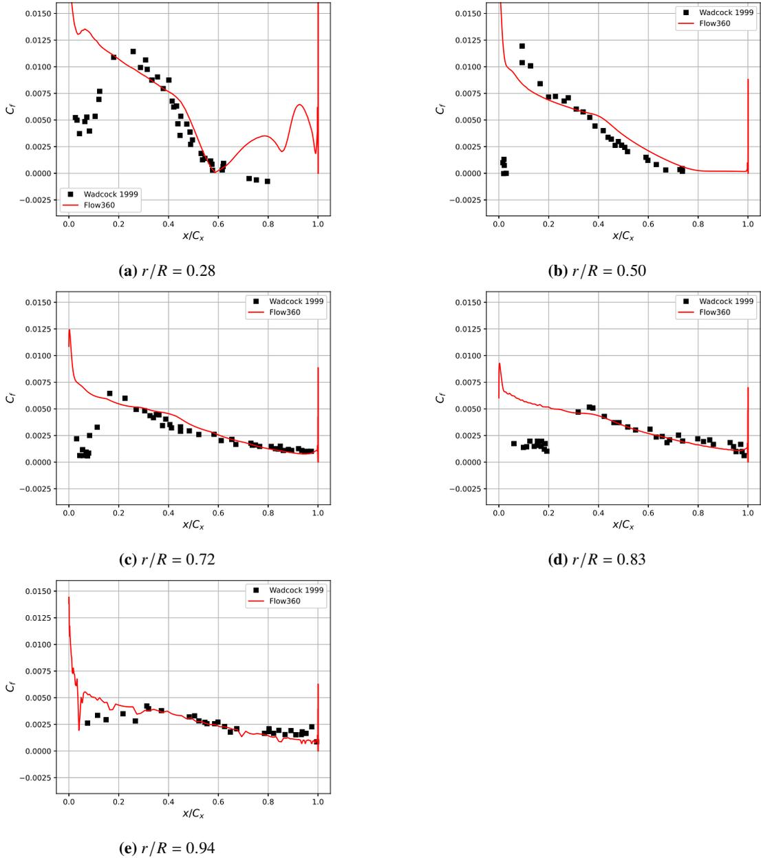
**Fig. 8 Comparison of predicted skin friction coefficient with the experimental data of Wadcock et al.[10]. Conditions employed:  $M_{tip} = 0.69$ ,  $Re = 4.95 \cdot 10^6$ , and  $\theta_{75} = 10^\circ$ .**
