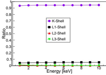
(a) The photoelectrons contribution from each shell in the case of using pure Ne for detection.
