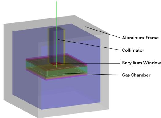
**Figure 1:** A simple GPD model in Geant4.
