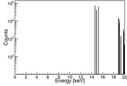
(b) The kinetic energy distribution of the emitted photoelectrons, in the case of injecting 20 keV photons into the GPD using pure Xe as working gas.
