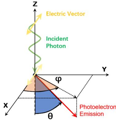
**Figure 6:** Schematic illustration of polarization detection for X-rays through the photoelectric effect. The exit direction of the photoelectron is mainly described by two angles, whereas the angle between the photoelectron and the incident photon is assigned as  $\theta$ , and the angle between the projection vector in the XY plane and the X-axis is described as  $\varphi$ .
