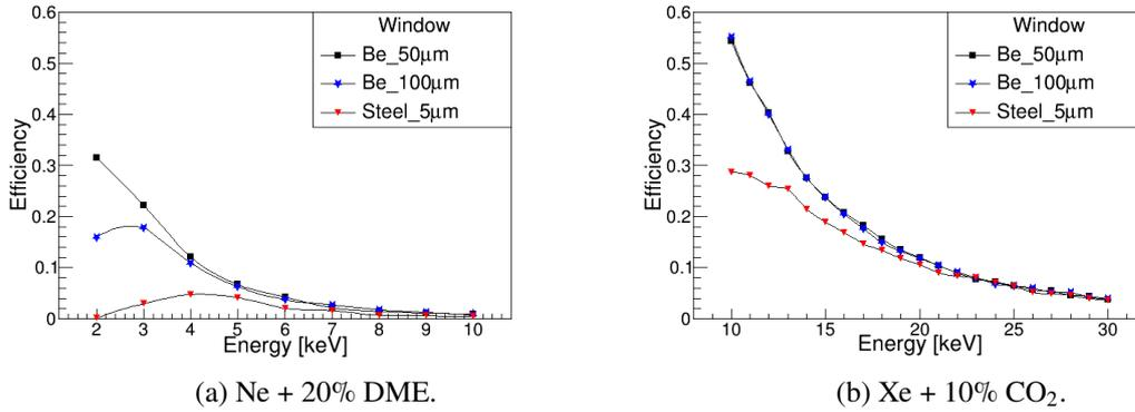
**Figure 4:** The detection efficiency of the Ne-based, and Xe-based GPD. As the energy increases, the detection efficiency decreases, but the Xe-based GPD still has a high detection efficiency at 10-30 keV.
