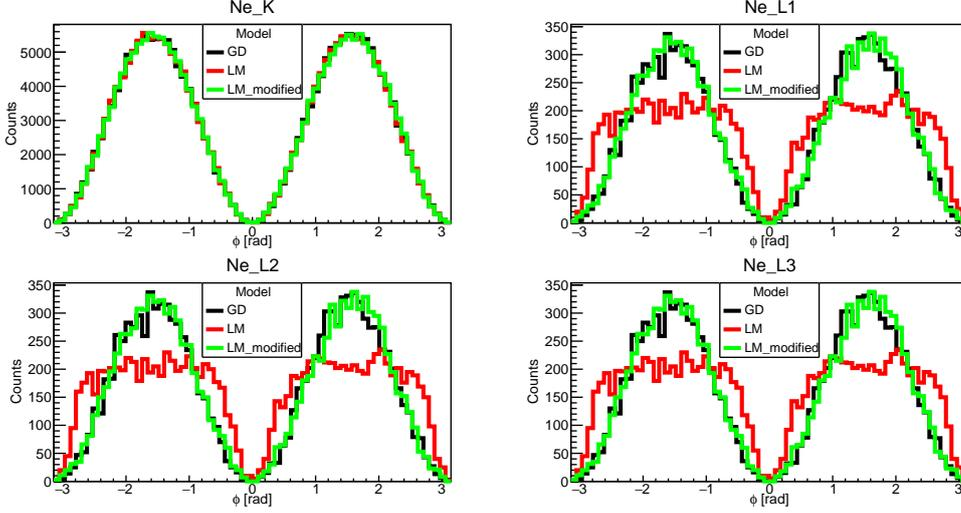
**Figure 9:** The emission angle ( $\varphi$ ) distribution of each bound shell (K, L1, L2, L3), in the case of injecting 8 keV linear polarization photons into the GPD using pure Ne as working gas. The simulation results of L shells using the LM model (red color) have serious distortions and their distributions are no longer a  $\cos^2 \varphi$  shape. The simulation results of the GD model and the LM\_modified model are in black and green color, respectively.
