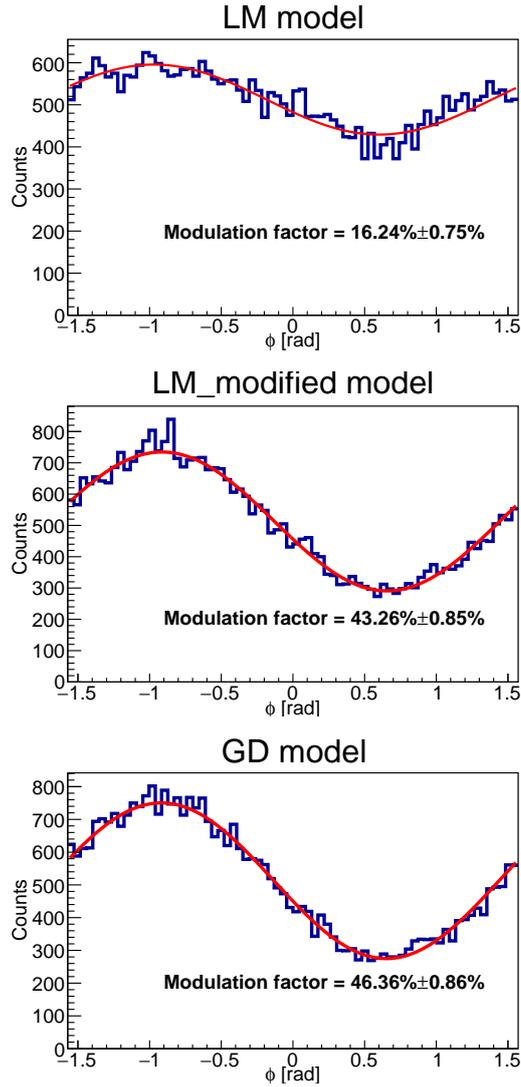
**Figure 11:** Reconstruction results of 20 keV photoelectron tracks simulated by different models.
