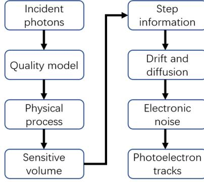
**Figure 2:** The process of simulating photoelectron tracks.
