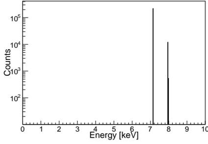
(a) The kinetic energy distribution of the emitted photoelectrons, in the case of injecting 8 keV photons into the GPD using pure Ne as working gas.
