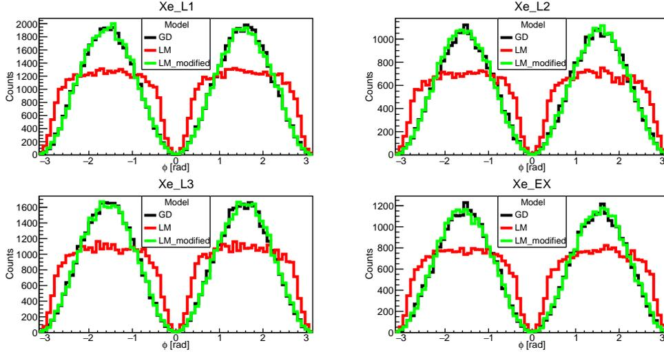
**Figure 10:** The emission angle ( $\varphi$ ) distribution of each bound shell (L1, L2, L3 and others shells), in the case of injecting 20 keV linear polarization photons into the GPD using pure Xe as working gas. The simulation results of L shells and higher shells using the LM model (red color) have serious distortions and their distributions are no longer a  $\cos^2 \varphi$  shape. The simulation results of the GD model and the LM\_modified model are in black and green color, respectively.
