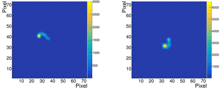
(a) An example of the simulated track in Ne-based GPD. (b) An example of the simulated track in Xe-based GPD.
