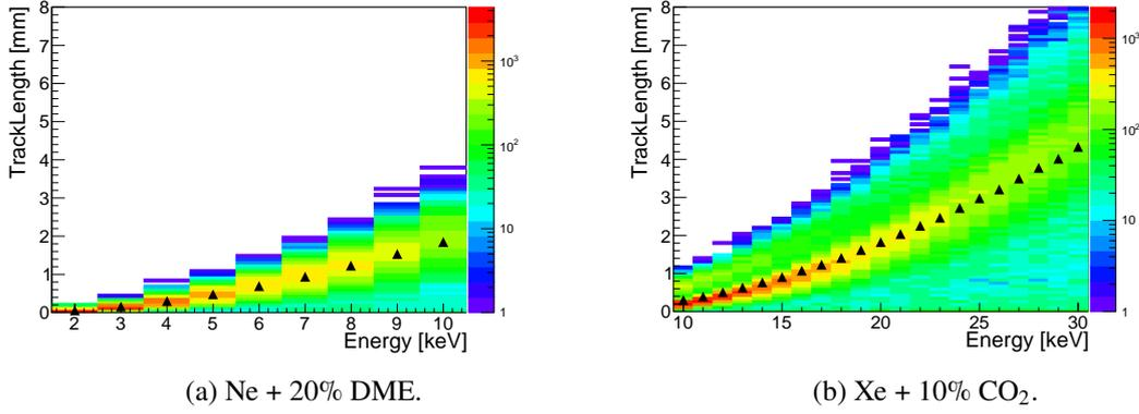
**Figure 5:** The distribution of photoelectron track length (on the two-dimensional image) versus X-ray photon energy. (a) The Ne-based GPD; (b) The Xe-based GPD. The black triangle is the average track length in specified X-ray energy.
