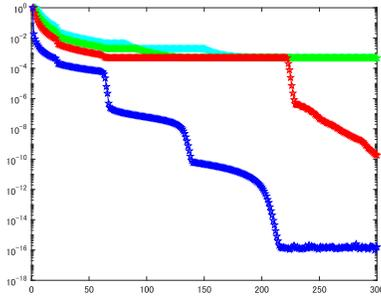
Figure 21:  $\frac{\sigma_k(H_{k+1,k})}{\sigma_1(H_{k+1,k})}$  (blue),  $\frac{\sigma_{k-1}(H_{k+1,k})}{\sigma_1(H_{k+1,k})}$  (red),  $\frac{\sigma_{k-2}(H_{k+1,k})}{\sigma_1(H_{k+1,k})}$  (green) and  $\frac{\sigma_{k-3}(H_{k+1,k})}{\sigma_1(H_{k+1,k})}$  (cyan) vs. number of iterations for GMRES using pseudoinverse for an inconsistent problem
