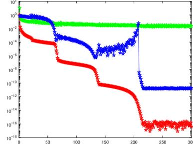
Figure 20:  $\frac{\|A^T \mathbf{r}_j\|_2}{\|A^T \mathbf{b}\|_2}$  (blue),  $\frac{\sigma_k(H_{k+1,k})}{\sigma_1(H_{k+1,k})}$  (red) and  $\frac{h_{j+1,j}}{\|H_{j,j}\|_F}$  (green) vs. number of iterations for GMRES using pseudoinverse and reorthogonalization for a range symmetric inconsistent problem
