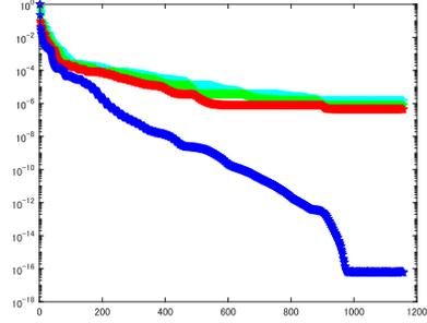
Figure 18:  $\frac{\sigma_k(H_{k+1,k})}{\sigma_1(H_{k+1,k})}$  (blue),  $\frac{\sigma_{k-1}(H_{k+1,k})}{\sigma_1(H_{k+1,k})}$  (red),  $\frac{\sigma_{k-2}(H_{k+1,k})}{\sigma_1(H_{k+1,k})}$  (green) and  $\frac{\sigma_{k-3}(H_{k+1,k})}{\sigma_1(H_{k+1,k})}$  (cyan) vs. number of iterations for GMRES using pseudoinverse and reorthogonalization for an inconsistent problem (**ex32**)
