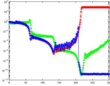
Figure 19:  $\frac{\|A^T \mathbf{r}_j\|_2}{\|A^T \mathbf{b}\|_2}$  vs. number of iterations for GMRES using pseudoinverse and reorthogonalization (blue), GMRES using reorthogonalization (red), and RRGMRES (green) for a range symmetric inconsistent problem
