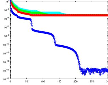
Figure 22:  $\frac{\sigma_k(H_{k+1,k})}{\sigma_1(H_{k+1,k})}$  (blue),  $\frac{\sigma_{k-1}(H_{k+1,k})}{\sigma_1(H_{k+1,k})}$  (red),  $\frac{\sigma_{k-2}(H_{k+1,k})}{\sigma_1(H_{k+1,k})}$  (green) and  $\frac{\sigma_{k-3}(H_{k+1,k})}{\sigma_1(H_{k+1,k})}$  (cyan) vs. number of iterations for GMRES using pseudoinverse and reorthogonalization for an inconsistent problem
