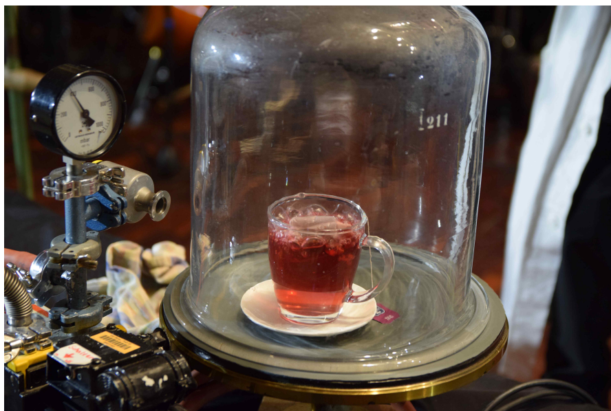
Figure 13: Vacuum chamber with pressure gauge at the back. The tea water is boiling as the pressure has been sufficiently lowered. The connection to the vacuum pump is below the saucer.
