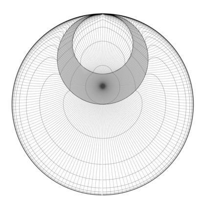
Fig. 1. Light rays and wavefronts emitted by a source of light refracting through a horizontal interface mapped to the Poincaré disc. The refractive index in the darker layer (where the light source is settled) is larger than the one in the whiter space.
