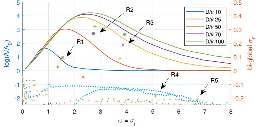
Figure 6: Mixing layer integrated spatial amplification factor compared to the global instability results. The asterisks indicate the global modes eigenvalues of Rossiter modes and the dots are other eigenvalues, and refer to the scale on the right hand side of the frame.
