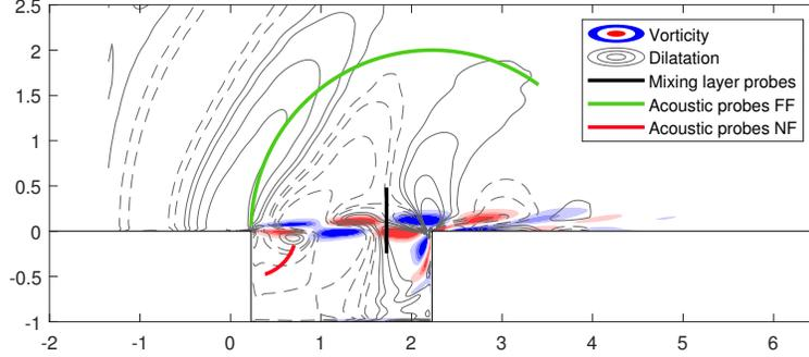
Figure 9: Location of probes for the analysis of sound emission. Gray contours indicate dilatation fluctuations of the second Rossiter mode at  $Ma = 0.6$ , full line for positive contours and dashed line for negative ones. Colored contours indicate vorticity fluctuations. The black line indicates region of evaluation of sound source magnitude. Red and green lines indicate regions of evaluation of the magnitude of the pressure fluctuations.
