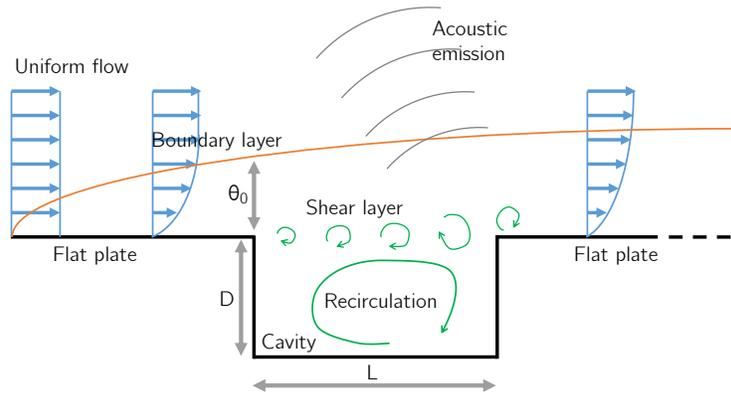
Figure 1: Illustration of the open cavity flow.
