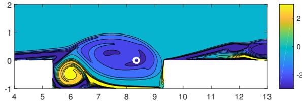
Figure 14: Vorticity contours of the unsteady flow at an arbitrary time. The white circle marks a point where data is collected for figure 15
