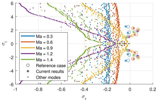
Figure 17: Eigenspectra computed for  $Ma = 0.3, 0.6, 0.9, 1.2$  and  $1.4$ , and comparison with reference values by Sun et al. [40].
