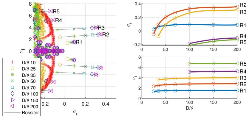
Figure 4: Eigenvalues from the  $D/\theta$  ratio sweep ( $Re_D = 1000$ ,  $Ma = 0.5$ ). (a) Eigen-spectrum. (b) Real and imaginary parts of Rossiter mode eigenvalues.
