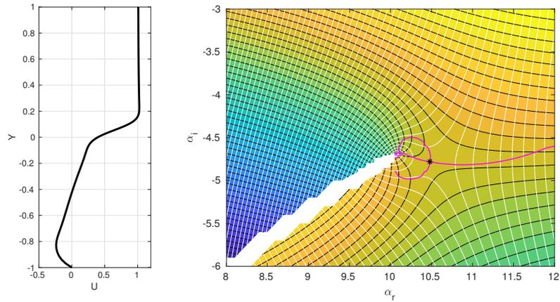
Figure 18: (a) Velocity profile considered for the absolute instability analysis. (b) Complex  $\omega$  mapped as a function of complex  $\alpha$ . The colors and black line contours indicate the imaginary part and the white lines, the real part. The magenta lines cross at the saddle point.
