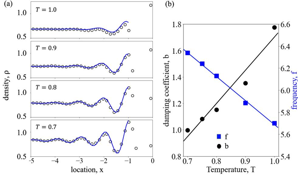
Figure 3: [Color online] (a) Oscillation of the intrinsic density profiles: circles denote results from MD simulations, solid lines are exponential fitting, as in Eq. (8), to the density profiles at different temperatures, (b) the damping coefficient (left  $y$  axis,  $\bullet$ ) increases with temperature, whereas, the frequency of oscillation (right  $y$  axis,  $\blacksquare$ ) decreases. The solid lines are linear fits to the data.
