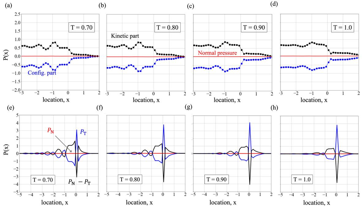
Figure 5: [Color online] (a-d) Constituent parts of the (—) normal component of pressure, i.e., (---) the kinetic part and, (---) the configurational part for (a)  $T = 0.70$ , (b)  $T = 0.80$ , (c)  $T = 0.90$  and, (d)  $T = 1.0$ . (e-h) Variation of (—) the tangential component of the pressure tensor and of (—)  $P_N - P_T$  near the interface for  $T = 0.70$  to 1.0.
