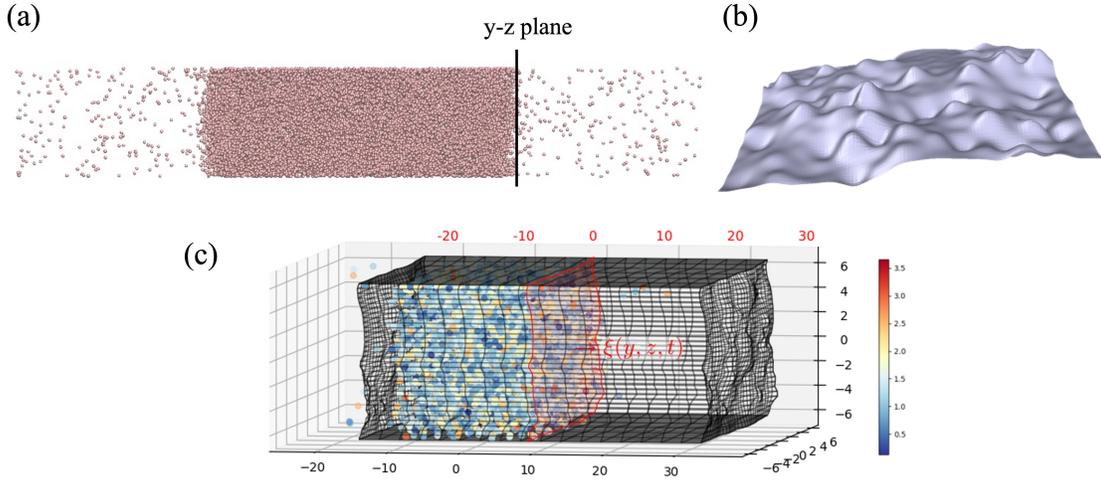
Figure 1: [Color online] (a) Liquid-vapor coexistence (b) fitted liquid-vapor surface function  $\xi$  ( $yz$  plane) (c) mapped grids at the interface,  $x = 0$  (mapped coordinates are in red at the top and un-mapped coordinates are in black at the bottom). The atoms are colored by their respective velocities, the bin-resolution is reduced here for visualization purpose. The mapping shifts every time the interface moves in the  $x$  direction.
