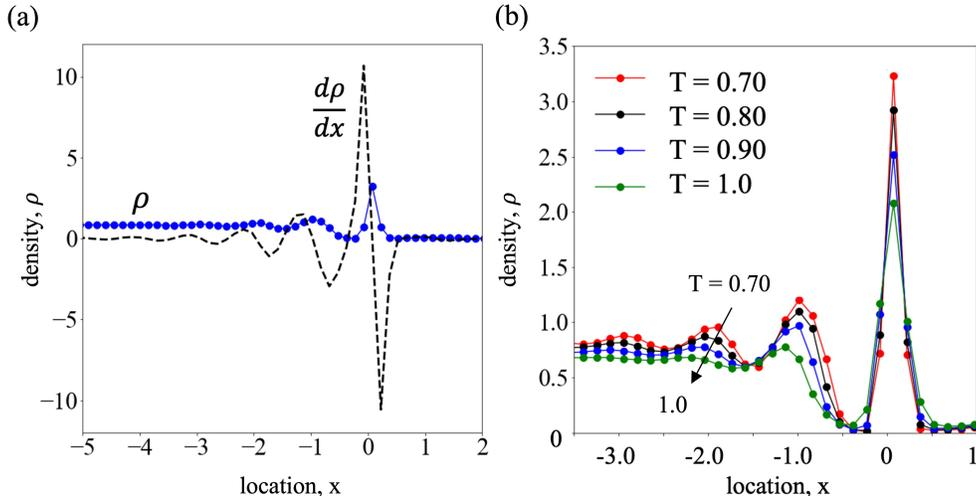
Figure 2: [Color online] (a) Density profile (blue circles) and derivative of density (black dashed line) for  $T = 0.70$  shows oscillations near the liquid-vapor interface (b) density profiles for a range of temperatures, oscillations are damped as temperature increases.
