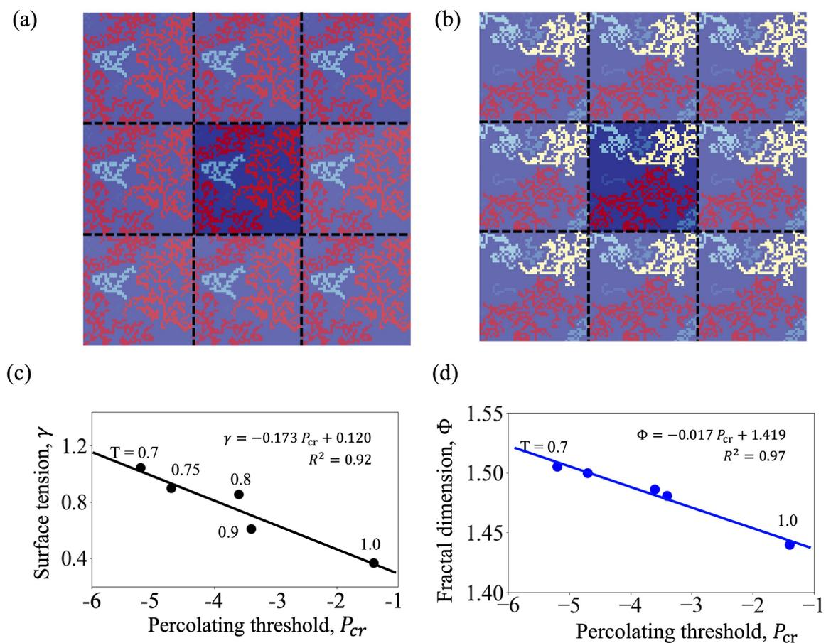
Figure 8: [Color online] Percolation network, with periodic images shown faintly, at a random instant at temperature (a)  $T = 0.8$  and, (b)  $T = 1.0$ . The largest cluster is colored red. Panel (a) shows a spanning cluster, whereas, in panel (b) no cluster is spanning throughout the surface for the same stress threshold. (c) Surface tension, and (d) fractal dimension as functions of the percolation threshold over the range of temperatures considered in this study, lines are linear fits.
