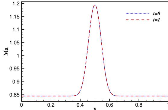
FIG. 5: Mach profile of the linear advection test at  $\delta t = 10^{-4}$ , using the *D2Q9* lattice,  $Nx = 400$  and  $\phi = 0$ .
