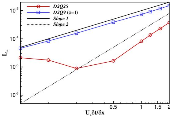
FIG. 6: Time refinement study in the simulation of advected vortex: convergence of the  $L_\infty$  error by decreasing the timestep.  $400 \times 400$  grid points are used.
