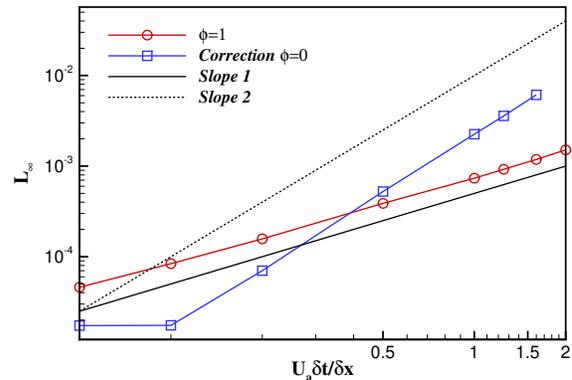
FIG. 7: Time refinement study in the simulation of advected vortex: convergence of the  $L_\infty$  error by decreasing the timestep. The  $D2Q9$  lattice is used with  $\phi = 1$  and  $\phi = 0$  augmented by the correction term.
