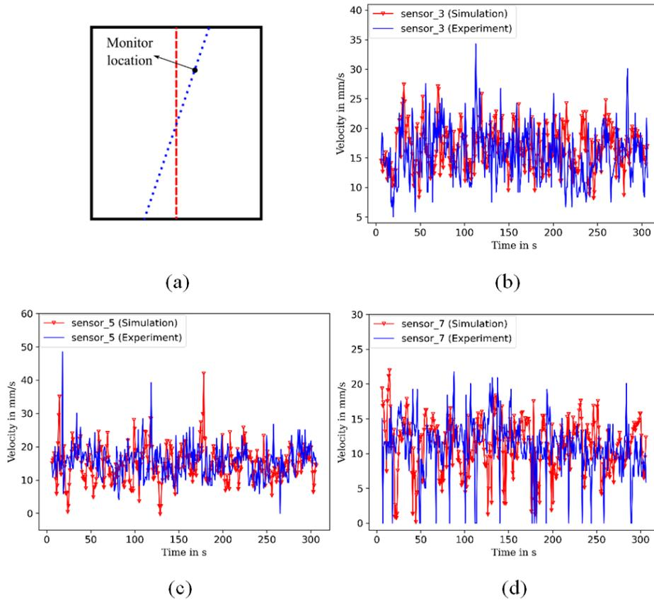
Figure 9: Comparisons of the time evolutions of the velocity on different UDV beam lines between numerical and experimental results (for  $b_z = -25.5 \mu\text{T}$ ): (a) Schematic diagram of the monitor location; (b) sensor 3; (c) sensor 5; (d) sensor 7.
