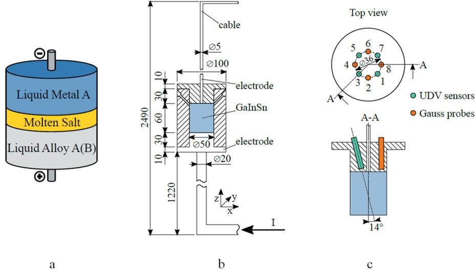
Figure 1: A schematic of an LMB (a), and the EVF experiment: (b) Sketch of the experiment. (c) Partially enlarged (1.5 : 1) cross-sectional view showing the distribution of the UDV sensors and the holes for the magnetic field measurements in more detail.
