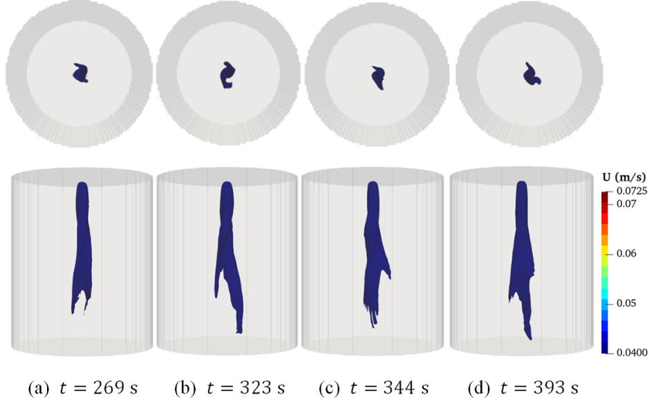
Figure 3: Iso-surface distributions of the higher transient velocity region ( $u \geq 0.04$  m/s) for  $b_z = -25.5 \mu\text{T}$  at different times. The bottom views are in the upper row, and the side views are in the lower row.
