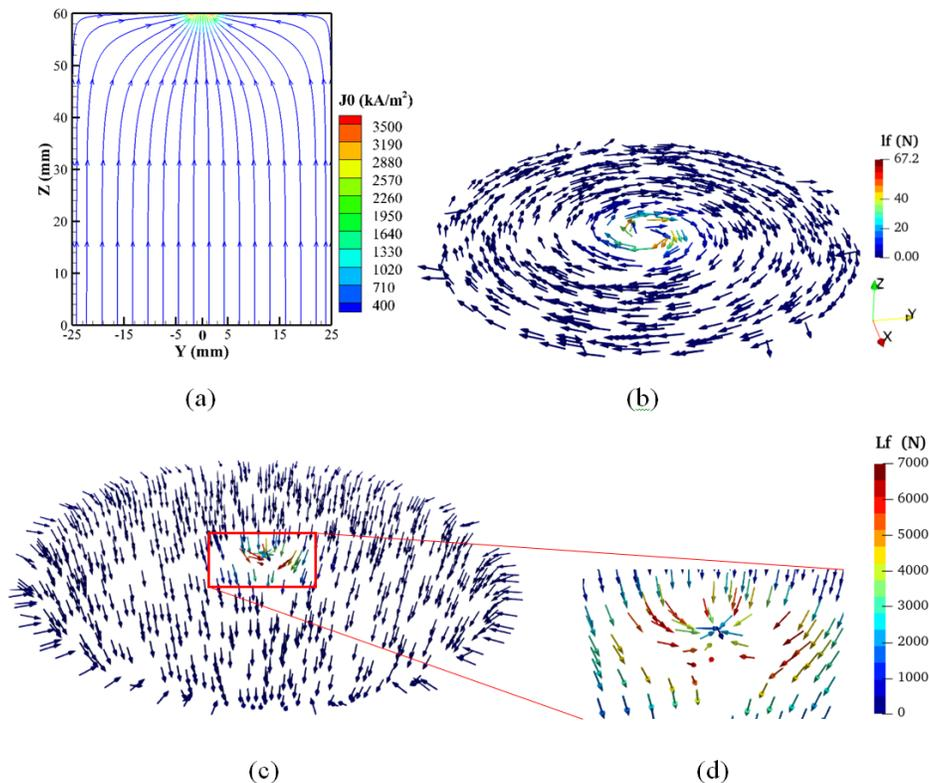
Figure 5: Distribution of (a) the imposed current density in the YOZ plane and Lorentz force on the  $z = 56$  mm cross-section for  $b_z = -25.5 \mu\text{T}$ : (b)  $\mathbf{J}_0 \times \mathbf{b}_z$ ; (c)  $\mathbf{J}_0 \times \mathbf{B}_0$ ; (d) partially enlarged view (2 : 1) of (c). Note the significant difference of the magnitudes between the two forces by a factor of approximately 100.
