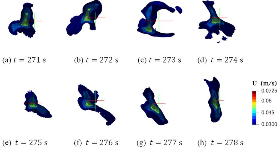
Figure 4: Top view of transient velocity iso-surface distribution below  $z = 30$  mm at different times at  $b_z = -25.5 \mu\text{T}$ , with  $u \geq 0.03$  m/s.
