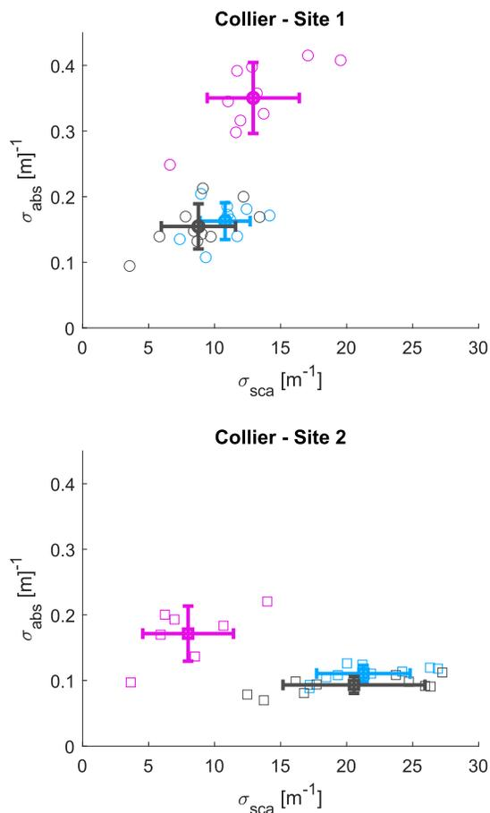
**Fig. 6.** Scattering and absorption coefficients from the two sites on Collier Glacier with black, cyan and magenta representing data taken at 405nm, 520nm and 640nm, respectively. Thick symbols are the mean scattering and absorption coefficient for each wavelength, and the error bars representing the standard deviation of each distribution.
