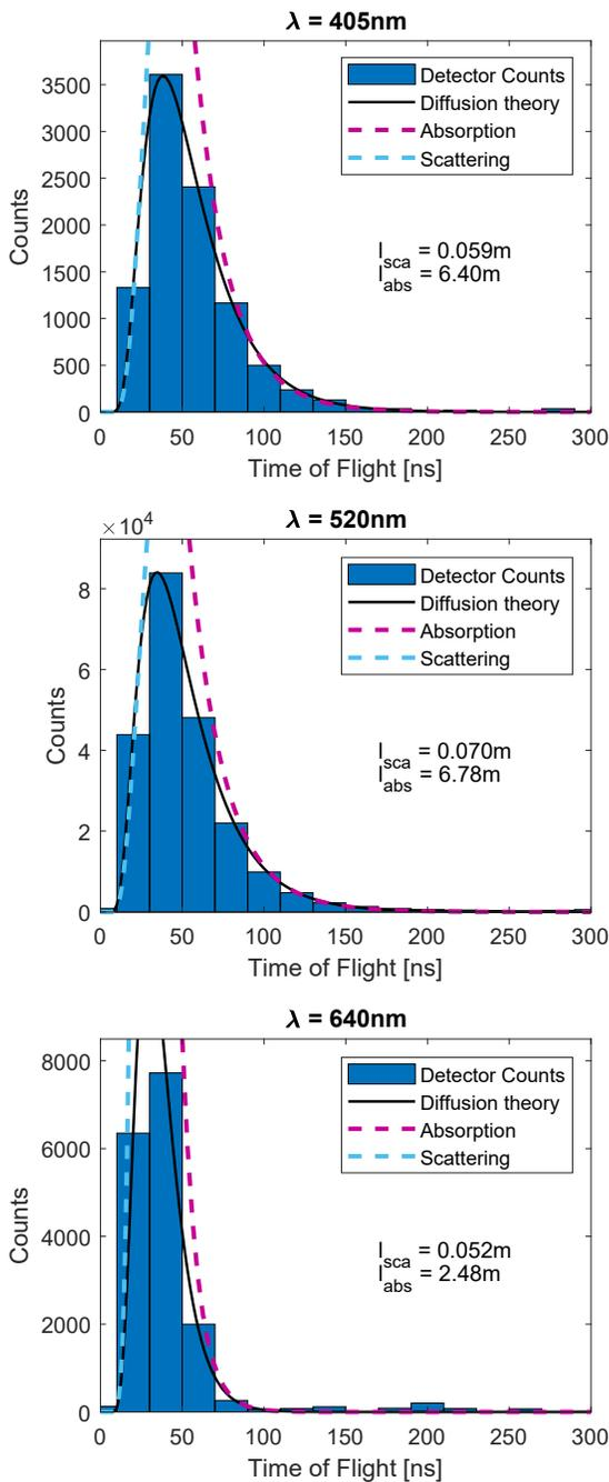
**Fig. 4.** Arrival-time histograms for the three different wavelength as recorded on Crook Glacier. Blue bars represent the background-subtracted data. The solid black line is the fitted diffusion curve, from which absorption and scattering coefficient are extracted. The cyan and magenta dashed lines are the diffusion curve with the absorptive and scattering component, respectively, turned off.
