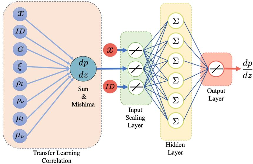
Figure 1: CoINN architecture components (left) it is the transfer learning component, the Sun & Mishima correlation, combined with the quality  $x$  and the inner diameter  $ID$  are the inputs of the ANN; (right) it comprises an input scaling layer, a hidden layer with 6 neurons, and  $\tanh$  as activation function and an output scaling layer.
