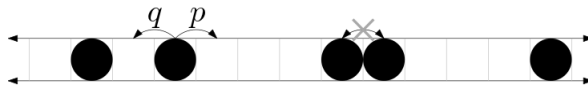
FIGURE 3. In the ASEP, particles jump left and right according to exponential clocks with rates q and p . All jumps are independent, and those that would lead to collisions are excluded (the grey \times ).
