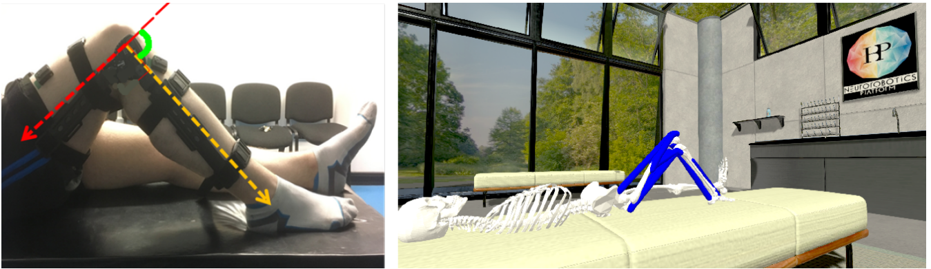
Figure 1. Human knee extension experiment: Participant Study with EMG recordings (Left) and experiment replication in the Neurorobotics Platform (Right).
