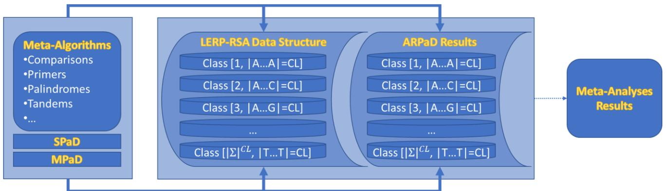
**Fig. 9** Execution of Meta-Analyses with Meta-Algorithms over the LERP-RSA and ARPaD results
