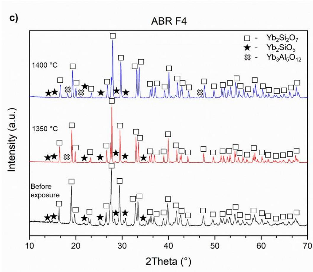
Figure 10: XRD measurements for a) EBC SG-100, b) ABR SG-100 and c) ABR F4. On each graph, bottom plot corresponds to the coating before steam exposure, middle to the 1350 °C steam exposure and top to the 1400 °C steam exposure. Phases have been identified with a square (□) for YbDS, a star (★) for YbMS and a cross (⊗) for the garnet
