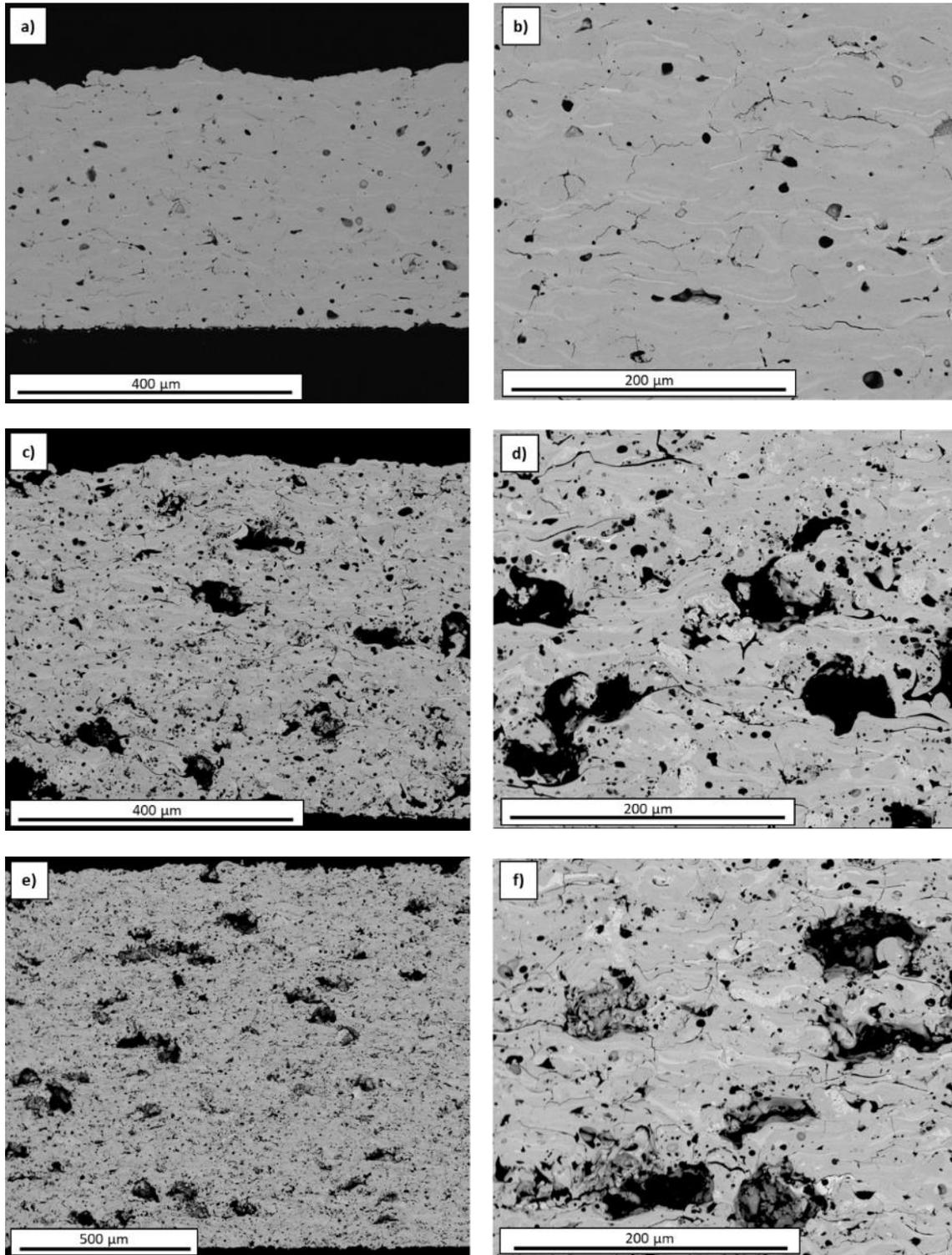
Figure 3: BSE images of the three free-standing coatings after annealing. Images a) and b) show sample EBC SG-100, c) and d) ABR SG-100 and e) and f) ABR F4
