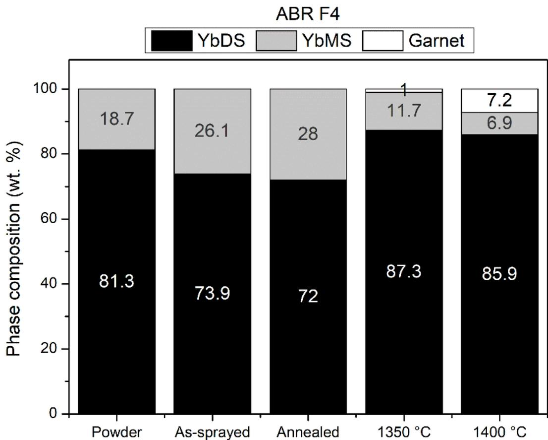
*Figure 11: Crystalline phase content quantified using Rietveld refinement for coatings EBC SG-100, ABR SG-100 and ABR F4*
