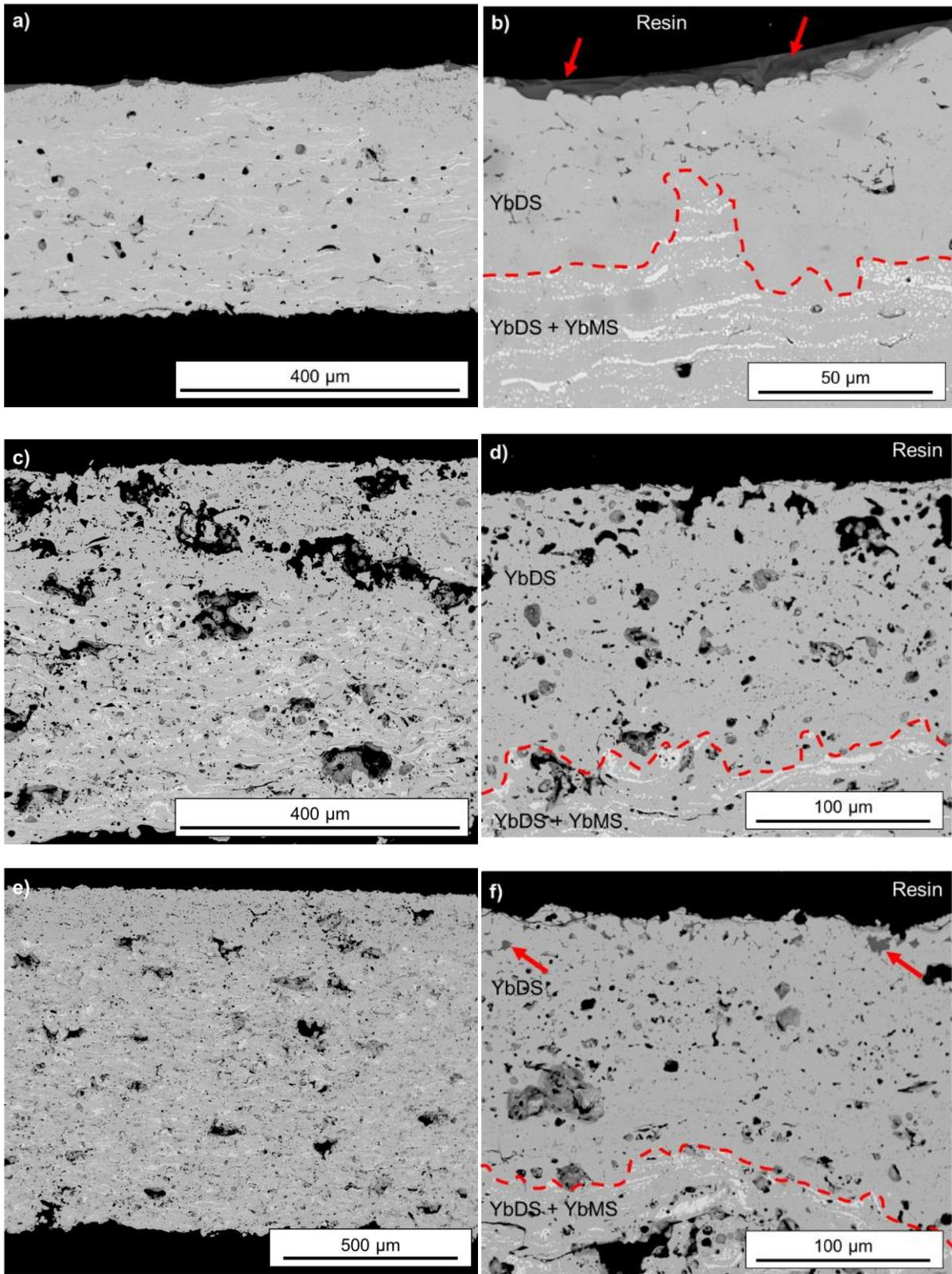
Figure 8: Low and high magnification BSE images of the cross-section of the samples exposed to steam for 96 h at 1400 °C. Images a) and b) correspond to sample EBC SG-100, images c) and d) to ABR SG-100 and images e) and f) to ABR F4. The red dashed line marks where no more YbMS could be found. Red arrows in images b) and f) indicate where a new phase was detected
