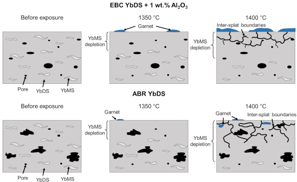
Figure 12: Schematic with the different behavior of EBC YbDS + 1 wt.% Al<sub>2</sub>O<sub>3</sub> and abrasible YbDS coatings when exposed to steam at high temperature
