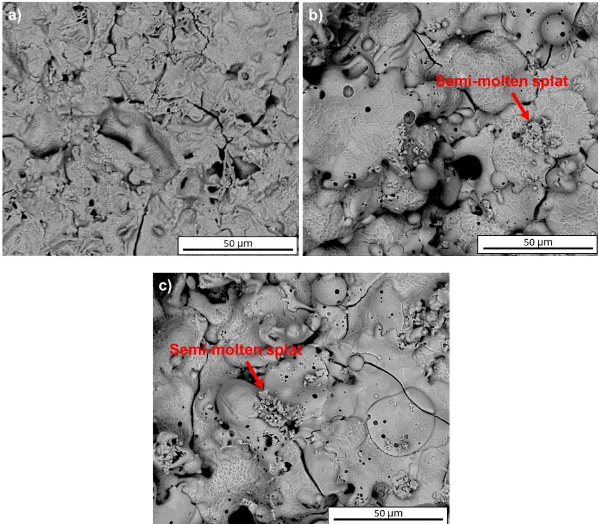
Figure 7: BSE images of the top surface of the samples exposed to steam at 1350 °C for 96 h. Image a) corresponds to sample EBC SG-100, image b) to ABR SG-100 and image c) to ABR F4
