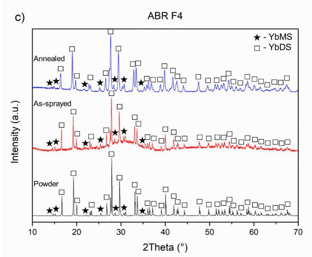
Figure 5: XRD measurements for a) EBC SG-100, b) ABR SG-100 and c) ABR F4. On each graph, the bottom plot corresponds to the powder, middle to the as-sprayed coating and top to the annealed coating. Phases have been identified with a star (★) for YbMS and a square (□) for YbDS
