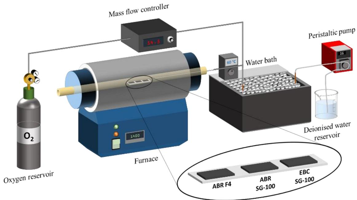
Figure 1: Schematic of the custom steam rig designed and built for the steam exposure
