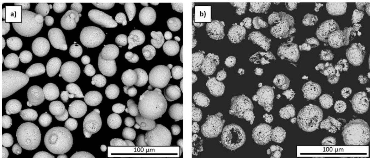
*Figure 2: BSE images of the powders used in this work: a) corresponds to sample EBC, b) corresponds to samples ABR*
