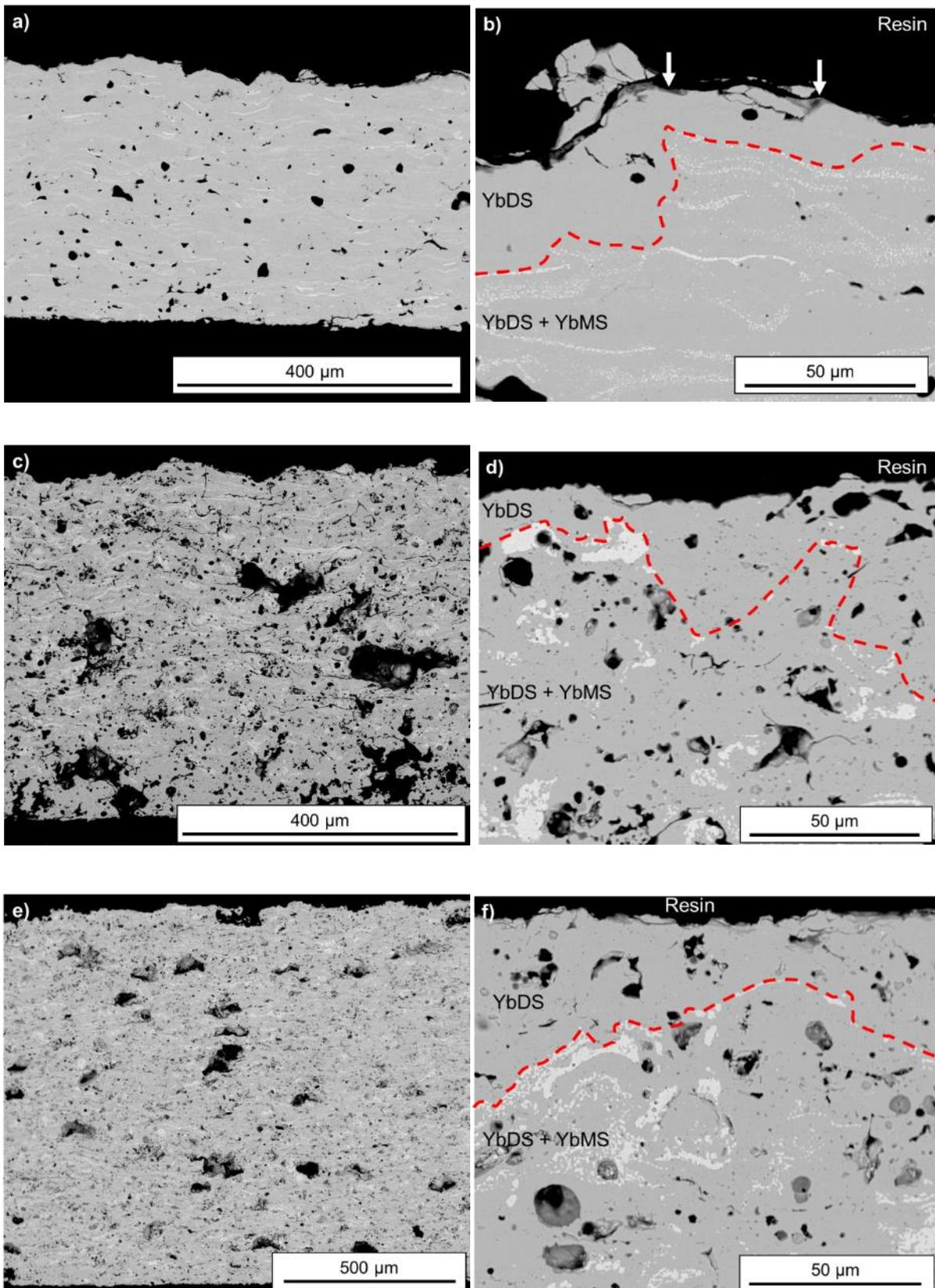
*Figure 6: Low and high magnification BSE images of the cross-section of the samples exposed to steam for 96 h at 1350 °C. Images a) and b) correspond to sample EBC SG-100, images c) and d) to ABR SG-100 and images e) and f) to ABR F4. The red dashed line marks where no more YbMS could be found. White arrows in image b) indicate where a new phase was detected*
