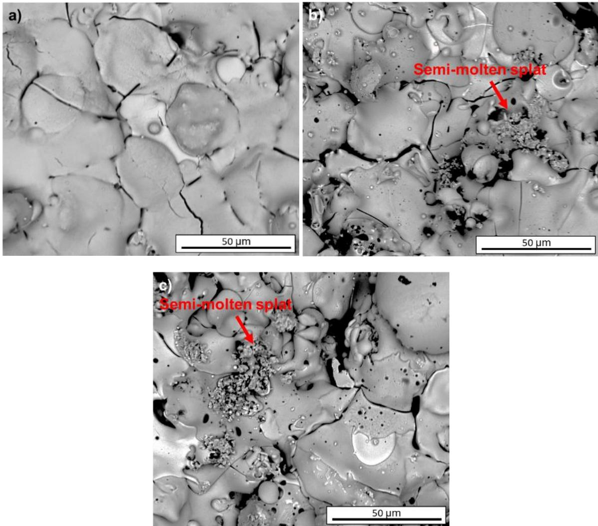
Figure 4: BSE images of the top surface of the annealed samples. Image a) corresponds to sample EBC SG-100, image b) to ABR SG-100 and image c) to ABR F4
