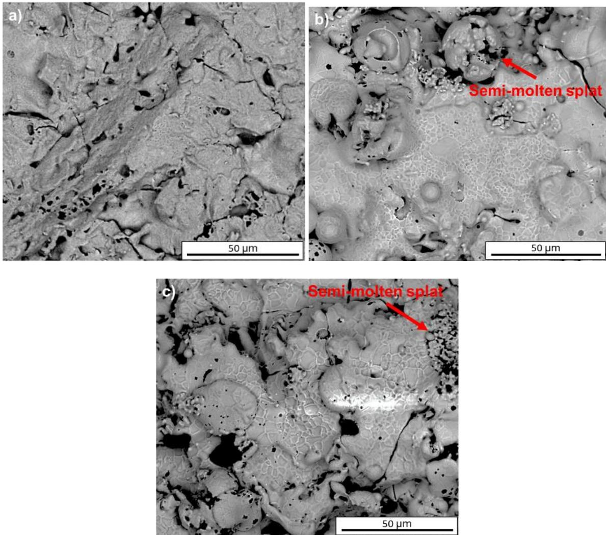
Figure 9: BSE images of the top surface of the samples exposed to steam at 1400 °C for 96 h. Image a) corresponds to sample EBC SG-100, image b) to ABR SG-100 and image c) to ABR F4
