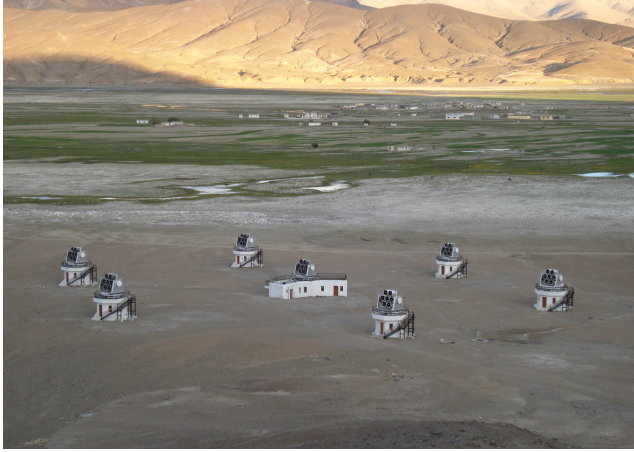
Fig. 6. 7-element HAGAR telescope array located at Hanle in India at an altitude of \sim 4.3 kms asl. Photo credit : HAGAR group
