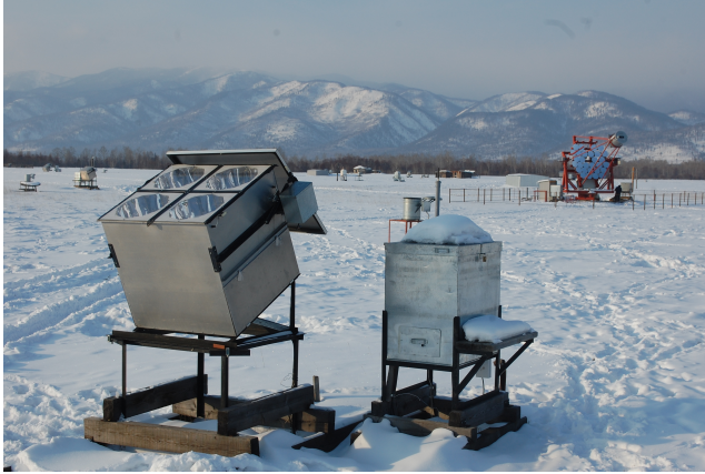
Fig. 23. One of the TAIGA-HiSCORE integrating Cherenkov detector stations with a wide Field of View is seen at the front in the above photograph. Each detector station consists of 4 large area PMTs. One installed TAIGA-IACT telescope seen at the back. Picture courtesy : TAIGA Collaboration.
